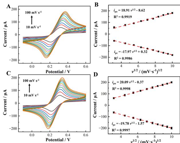
**Fig. 3** CV curves of (A) LIG and (B) rGO-LIG with different scan rates in 0.1 M KCl solution containing 5 mM  $[\text{Fe}(\text{CN})_6]^{3-/4-}$ ; (C) LIG and (D) rGO-LIG peak current as a function of the square root of the scan.
