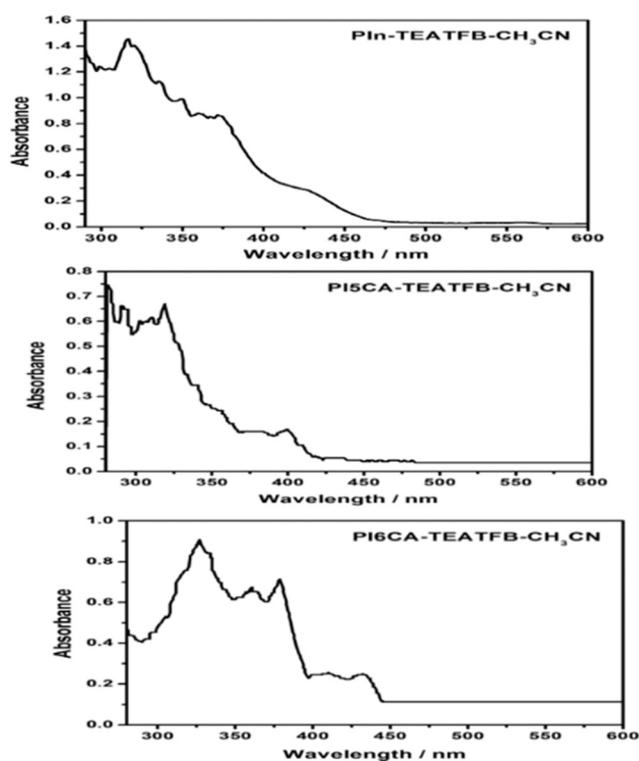
Fig. 4 UV-vis spectra of polyindole made from P5CA as PI5CA and I6CA as PI6CA in DMSO.
