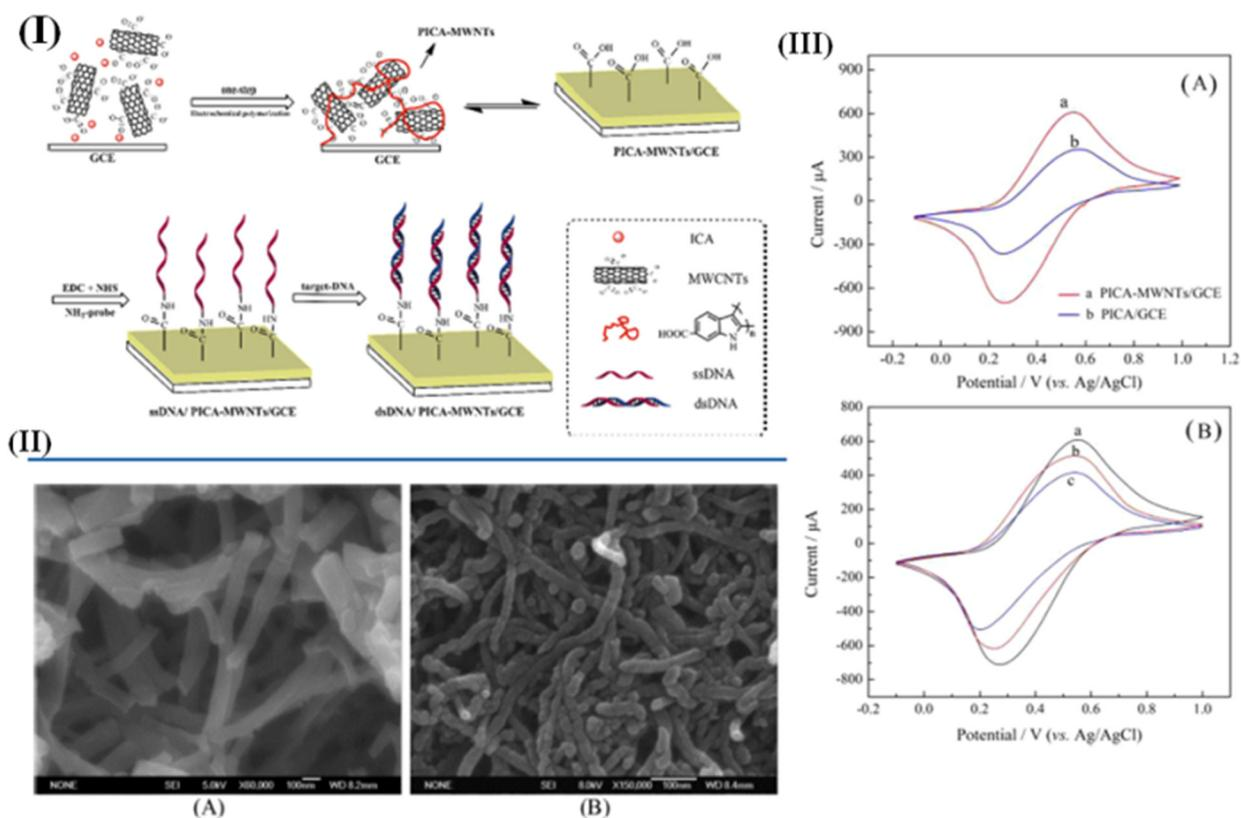
**Fig. 14** (I) Preparations of PICA-MWNT composite material and the corresponding conceptual scheme for label-free DNA detection, (II) SEM of PICA film (A) and PICA-MWNT composite film (B) deposited on GCE and (III) CVs of (A) PICA-MWNT (a) and pure PICA film (b); (B) PICA-MWNT (a), ssDNA/PICA-MWNT (b), and dsDNA/PICA-MWNT (c) in NaAc-HAc buffer (pH = 6.5, 0.1 mol L<sup>-1</sup> NaCl). Scan rate: 100 mV s<sup>-1</sup>. Reproduced with permission,<sup>84</sup> © ACS 2012.
