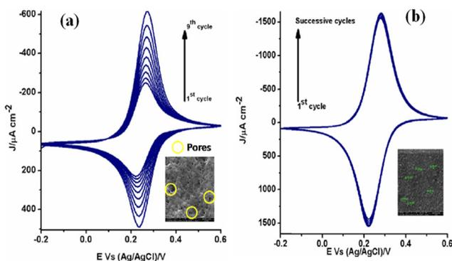
Fig. 12 (a) Cyclic voltammogram of siloxane-Au<sub>sim</sub> NPs showing increasing current trend at a scan rate of 10 mV s<sup>-1</sup> (b) cyclic voltammogram of Au@siloxane<sub>homo</sub> current with successive cycles at a scan rate of 10 mV s<sup>-1</sup>. Inset showing TEM micrographs of siloxane immobilized AuNPs (siloxane-Au<sub>sim</sub> NPs).
