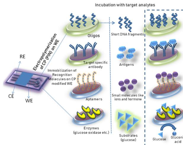
Fig. 13 CP based biosensors. Immobilization of recognition elements and binding of target molecules.
