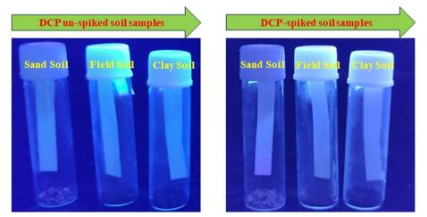
Fig. 10 Pictorial representation of soil sample observation before and after exposure to DCP vapor under UV light irradiation.
