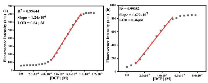
Fig. 6 Estimation of LOD and LOQ by plotting [DCP] vs. fluorescence intensity in (a) pure DMSO and (b) 50% (v/v) water-DMSO medium, respectively.
