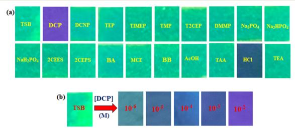
Fig. 8 (a) Response of TSB-coated filter paper strips towards DCP and other analyte solutions was observed upon exposure to a 365 nm UV lamp. (b) Fluorimetric color change of TSB-coated test kits across numerous concentrations ( $10^{-6}$  M to  $10^{-2}$  M) of DCP.
