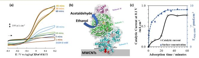
Fig. 2 (a) Cyclic voltammograms at PQQ-ADH/MWCNTs-modified GCE in 0.1 M acetate buffer solution (pH 5.5) containing  $CaCl_2$  in the presence of 0.1 M ethanol at a scan rate of 10 mV s<sup>-1</sup> under an argon atmosphere for various PQQ-ADH modification times; (b) illustration of DET between PQQ-ADH and the MWCNTs surface; <sup>30,31,34,50</sup> (c) catalytic oxidation current, PQQ-ADH surface concentration, PQQ-ADH layer number as a function of PQQ-ADH modification time.
