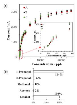
Fig. 4 (a) Sensitivity of CNF film sensor from triplicate amperometry measurements (marked as A-C). The insert zooms in parts for lower ethanol gas concentrations. (b) Selectivity of CNF film sensor as relative response compared to the ethanol gas.
