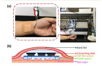
Fig. 6 (a) Photograph of non-invasive ethanol gas detection, and (b) illustration of a skin gas monitoring system.
