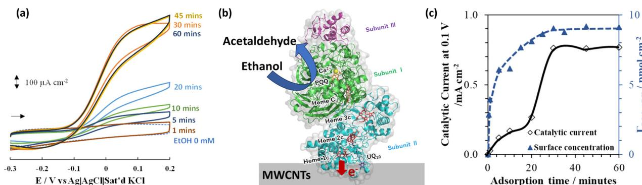
Fig. 2 (a) Cyclic voltammograms at PQQ-ADH/MWCNTs-modified GCE in 0.1 M acetate buffer solution (pH 5.5) containing  $\text{CaCl}_2$  in the presence of 0.1 M ethanol at a scan rate of  $10 \text{ mV s}^{-1}$  under an argon atmosphere for various PQQ-ADH modification times; (b) illustration of DET between PQQ-ADH and the MWCNTs surface;<sup>30,31,34,50</sup> (c) catalytic oxidation current, PQQ-ADH surface concentration, PQQ-ADH layer number as a function of PQQ-ADH modification time.
