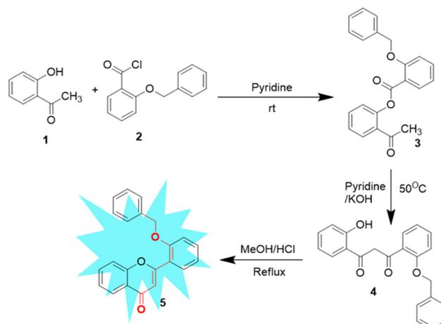
Scheme 2 Synthesis of the fluorophore, 2'-benzyloxy flavone.
