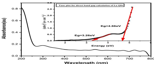
Fig. 10 UV-visible spectra with the Tauc plot of La QDs.
