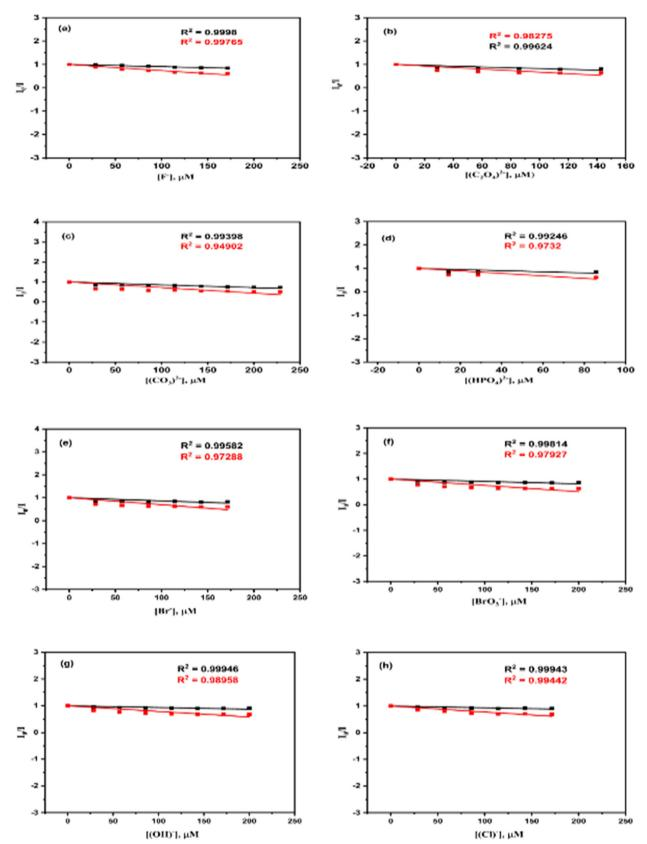
Fig. 17 Stern–Volmer plots for various sensors at 315 and 440.5 nm wavelengths: (a)  $F_{-}$ , (b)  $C_{2}O_{4}^{2-}$ , (c)  $CO_{3}^{2-}$ , (d)  $HPO_{4}^{2-}$ , (e)  $Br_{-}^{7}$ , (f)  $BrO_{3}^{-}$ , (g)  $OH_{-}^{7}$ , and (h) Cl<sup>-</sup>.
