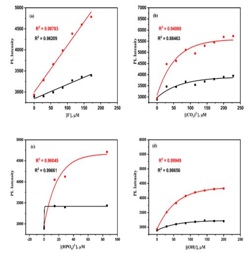
Fig. 16 Calibration curves for various sensors at 315 and 440.5 nm wavelengths: (a) F<sup>-</sup>, (b) CO<sub>3</sub><sup>2-</sup>, (c) HPO<sub>4</sub><sup>2-</sup>, and (d) OH<sup>-</sup>.
