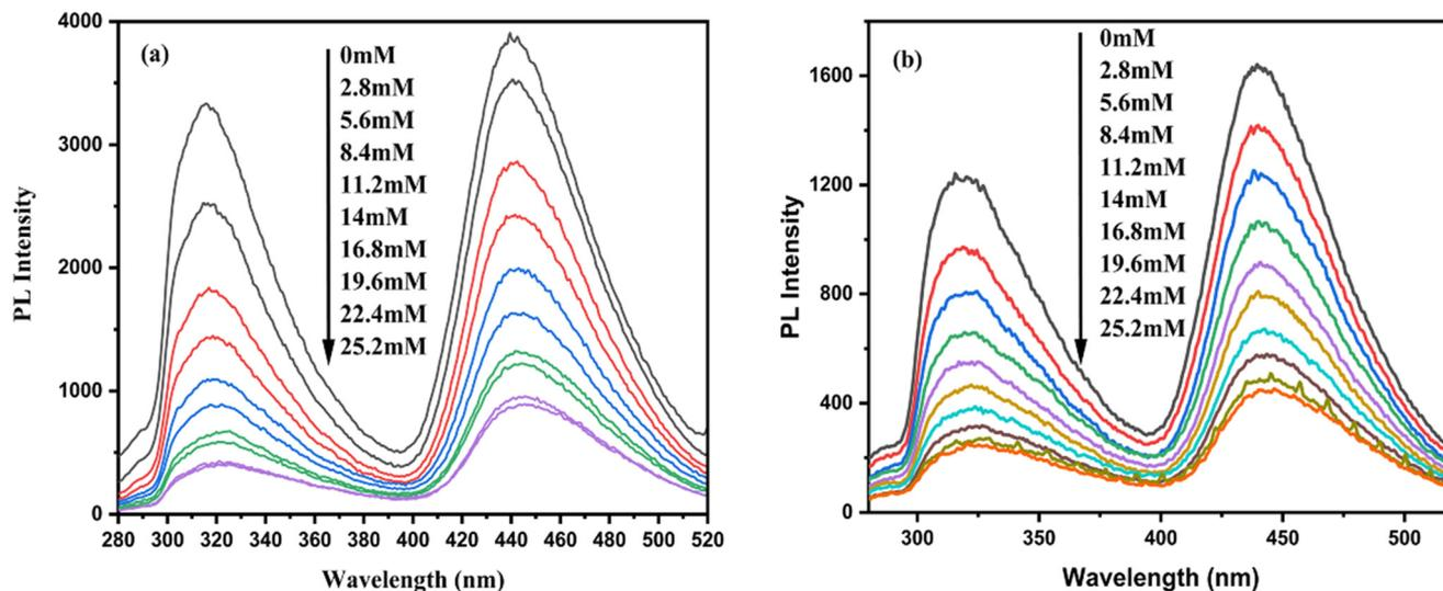
Fig. 19 Emission spectra of the optical La QD sensor under different [H<sub>2</sub>O<sub>2</sub>] at 315 nm and 440.5 nm wavelengths: (a) at room temperature, and (b) at 40 °C.
