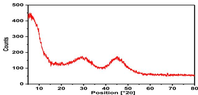
**Fig. 1** XRD pattern of the synthesized La QDs.
