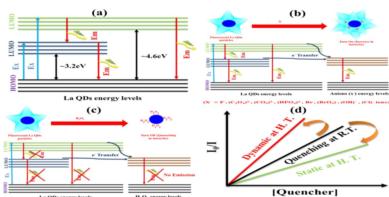
Fig. 14 Schematic of the fluorescence mechanism of (a) La QDs in sensing (b) anions and (c)  $\text{H}_2\text{O}_2$ . (d) Comparison between static and dynamic quenching.
