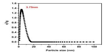
Fig. 9 Density distribution spectra of La QDs.
