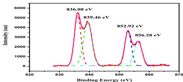
**Fig. 3** La 3d high-resolution XPS pattern of the synthesized La QDs.
