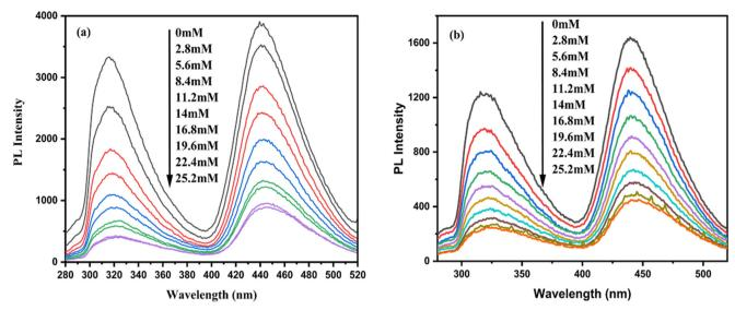
Fig. 19 Emission spectra of the optical La QD sensor under different  $[H_2O_2]$  at 315 nm and 440.5 nm wavelengths: (a) at room temperature, and (b) at 40 °C.
