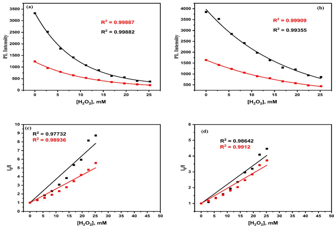
Fig. 20 Calibration curves of H<sub>2</sub>O<sub>2</sub> sensor peaks at: (a) 315 nm, and (b) 440.5 nm wavelengths. Stern-Volmer plots of H<sub>2</sub>O<sub>2</sub> sensor peaks at: (c) 315 nm, and (d) 440.5 nm wavelengths.
