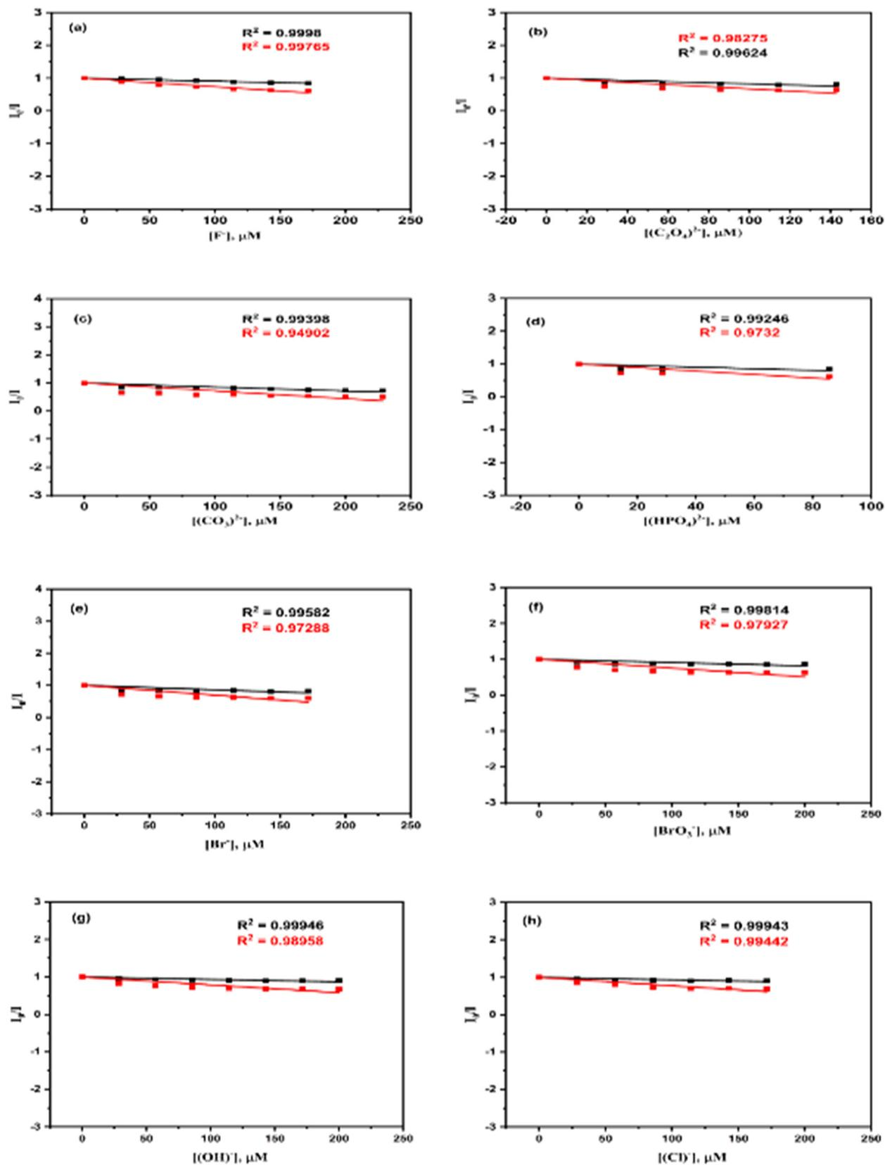
Fig. 17 Stern-Volmer plots for various sensors at 315 and 440.5 nm wavelengths: (a)  $F^-$ , (b)  $C_2O_4^{2-}$ , (c)  $CO_3^{2-}$ , (d)  $HPO_4^{2-}$ , (e)  $Br^-$ , (f)  $BrO_3^-$ , (g)  $OH^-$ , and (h)  $Cl^-$ .
