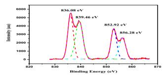
Fig. 3 La 3d high-resolution XPS pattern of the synthesized La QDs.
