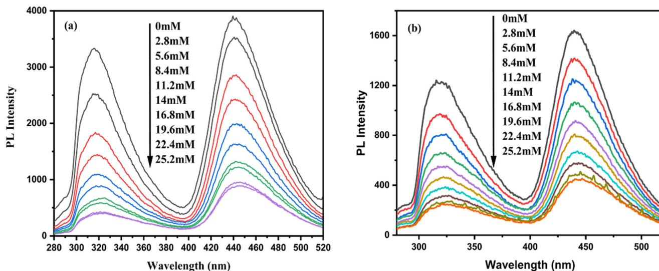
Fig. 19 Emission spectra of the optical La QD sensor under different  $[\text{H}_2\text{O}_2]$  at 315 nm and 440.5 nm wavelengths: (a) at room temperature, and (b) at 40 °C.
