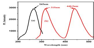
Fig. 11 (a) Excitation spectra of the La QDs in ethanol with a maximum emission at 315 nm wavelength. (b) Emission spectra of the La QDs in ethanol with an excitation at 265 nm wavelength.
