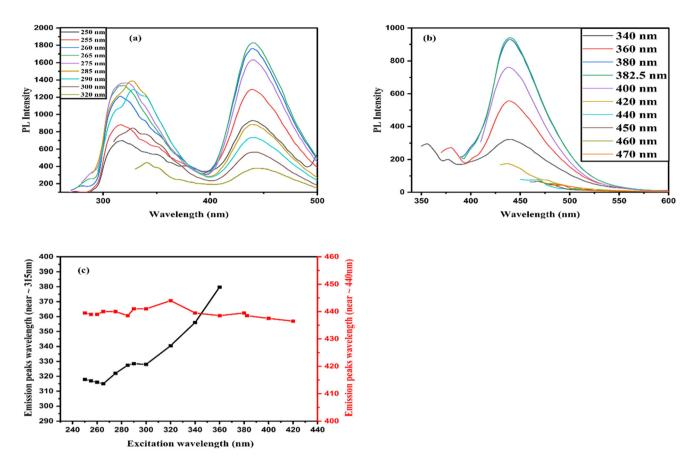
Fig. 13 PL spectra of La QDs obtained (a) at nine distinct excitation wavelengths between 250 and 320 nm and (b) at ten distinct excitation wavelengths between 340 and 470 nm. (c) PL peak position of La QDs concerning the excitation wavelength.
