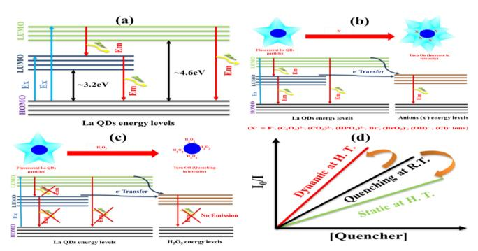
Fig. 14 Schematic of the fluorescence mechanism of (a) La QDs in sensing (b) anions and (c) H<sub>2</sub>O<sub>2</sub>. (d) Comparison between static and dynamic quenching.
