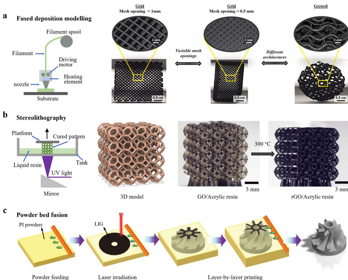
**Fig. 2** 3D printing of graphene. (a) Different architectures by fused deposition modelling. The printing direction affects graphene's properties. Reproduced from ref. 121 under creative commons CC-BY license. (b) Graphene cell printed by stereolithography. Reproduced from ref. 125 with permission from Wiley-VCH GmbH, copyright 2023. (c) Sophisticated graphene devices printed with a modified powder bed fusion method. Reproduced from ref. 126 under creative commons CC-BY license.
