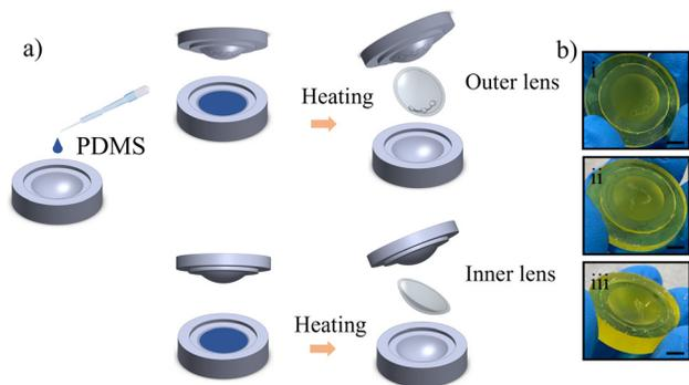
**Fig. 1** Fabrication process of both inner and outer layers of the contact lens. a) Contact lens molding and b) 3D printed contact lens molds: i) male mold containing a microfluidic channel (scale bar 4 mm), ii) male mold (scale bar 3 mm) and iii) female mold (scale bar 5 mm).
