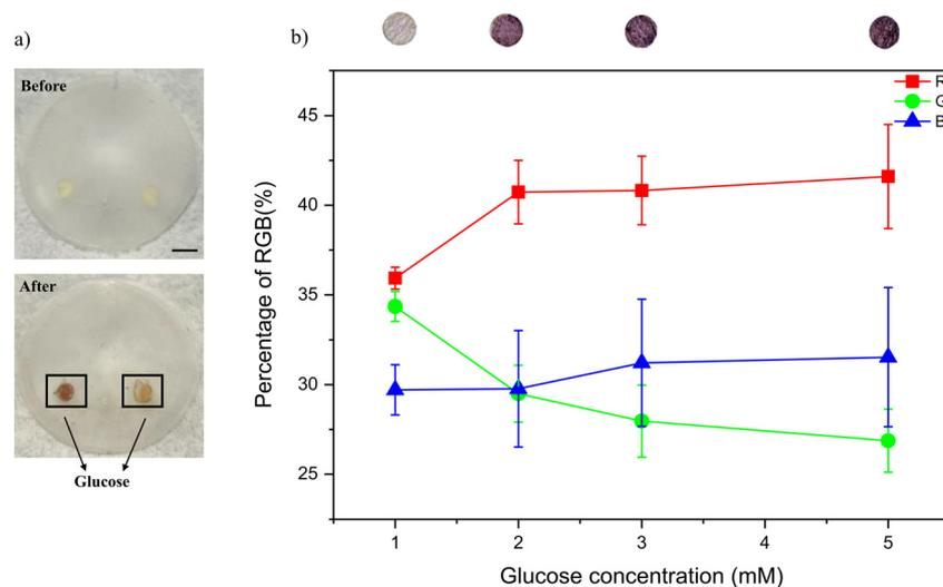
**Fig. 4** a) Photo of the paper integrated contact lens before glucose introduction and after glucose introduction. b) RGB percentage with respect to glucose concentration. Decreasing G level indicates increasing glucose concentration.
