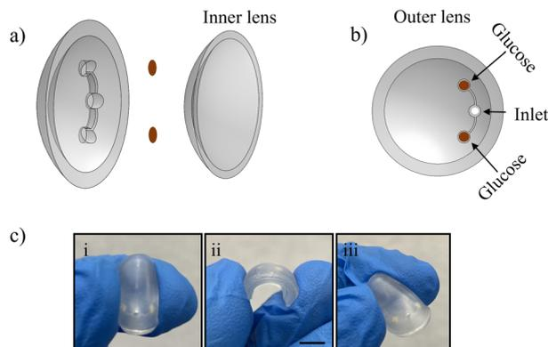
**Fig. 2** Schematic illustration of different layers of the SCL. a) Schematic of the microfluidic contact lens, b) inner side of the outer lens and c) contact lens under mechanical stress, bending, and from different angles (i-iii).
