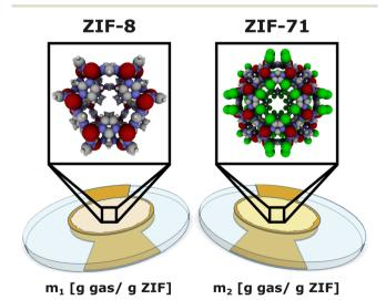
Fig. 1 Sensor array design. Our proposed gas sensor array design is comprised of two distinct QCM-ZIF sensors, one employing a ZIF-8 sensing film, the other ZIF-71. The sensor array response vector is  $\mathbf{m} =$  $[m_{\rm ZIF-8},\ m_{\rm ZIF-71}]$  where  $m_{\rm ZIF-\it{i}}$  is the total mass of gas adsorbed in ZIF- $\it{i}$ film per mass of ZIF, at thermodynamic equilibrium.
