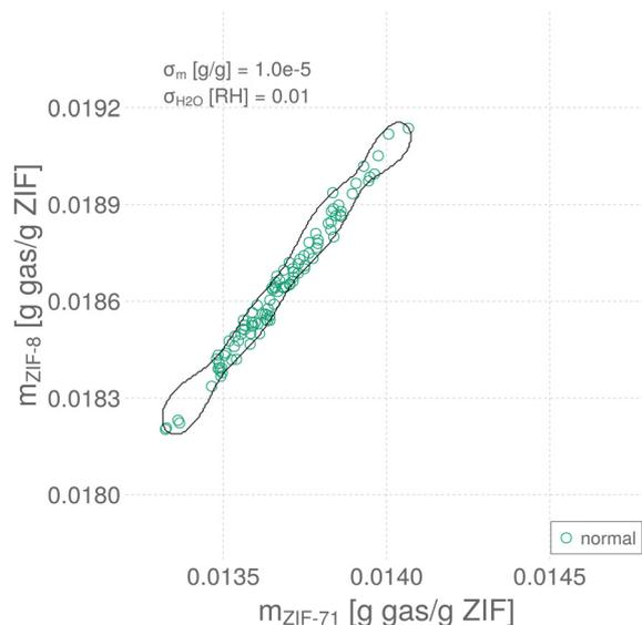
**Fig. 4** Training an SVDD anomaly detector. A synthetic data set ( $\{m_i, \text{normal}\}$ ) of sensor array response vectors collected under normal conditions in the ripening room and the decision boundary of the SVDD trained on it (optimal  $\nu = 0.012$ ,  $\gamma = 0.540$ ).
