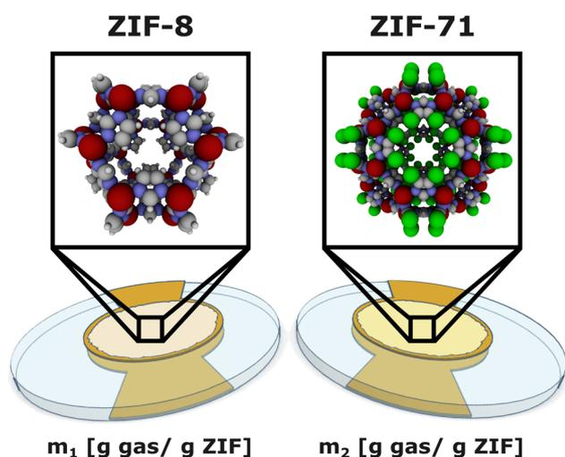
**Fig. 1** Sensor array design. Our proposed gas sensor array design is comprised of two distinct QCM-ZIF sensors, one employing a ZIF-8 sensing film, the other ZIF-71. The sensor array response vector is  $\mathbf{m} = [m_{\text{ZIF-8}}, m_{\text{ZIF-71}}]$  where  $m_{\text{ZIF-}i}$  is the total mass of gas adsorbed in ZIF- $i$  film per mass of ZIF, at thermodynamic equilibrium.
