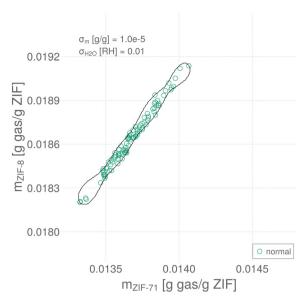
Fig. 4 Training an SVDD anomaly detector. A synthetic data set {(m<sub>i</sub>, normal)} of sensor array response vectors collected under normal conditions in the ripening room and the decision boundary of the SVDD trained on it (optimal v = 0.012,  $\gamma = 0.540$ ).
