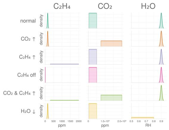
Fig. 2 Gas compositions we expect to encounter in a fruit ripening room. The probability distributions of the  $C_2H_4$ ,  $CO_2$ , and  $H_2O$  concentrations (columns) in the air of a fruit ripening room under normal and various anomalous conditions (rows). RH = relative humidity.  $\sigma_{H_2O}$  = 0.01 RH.
