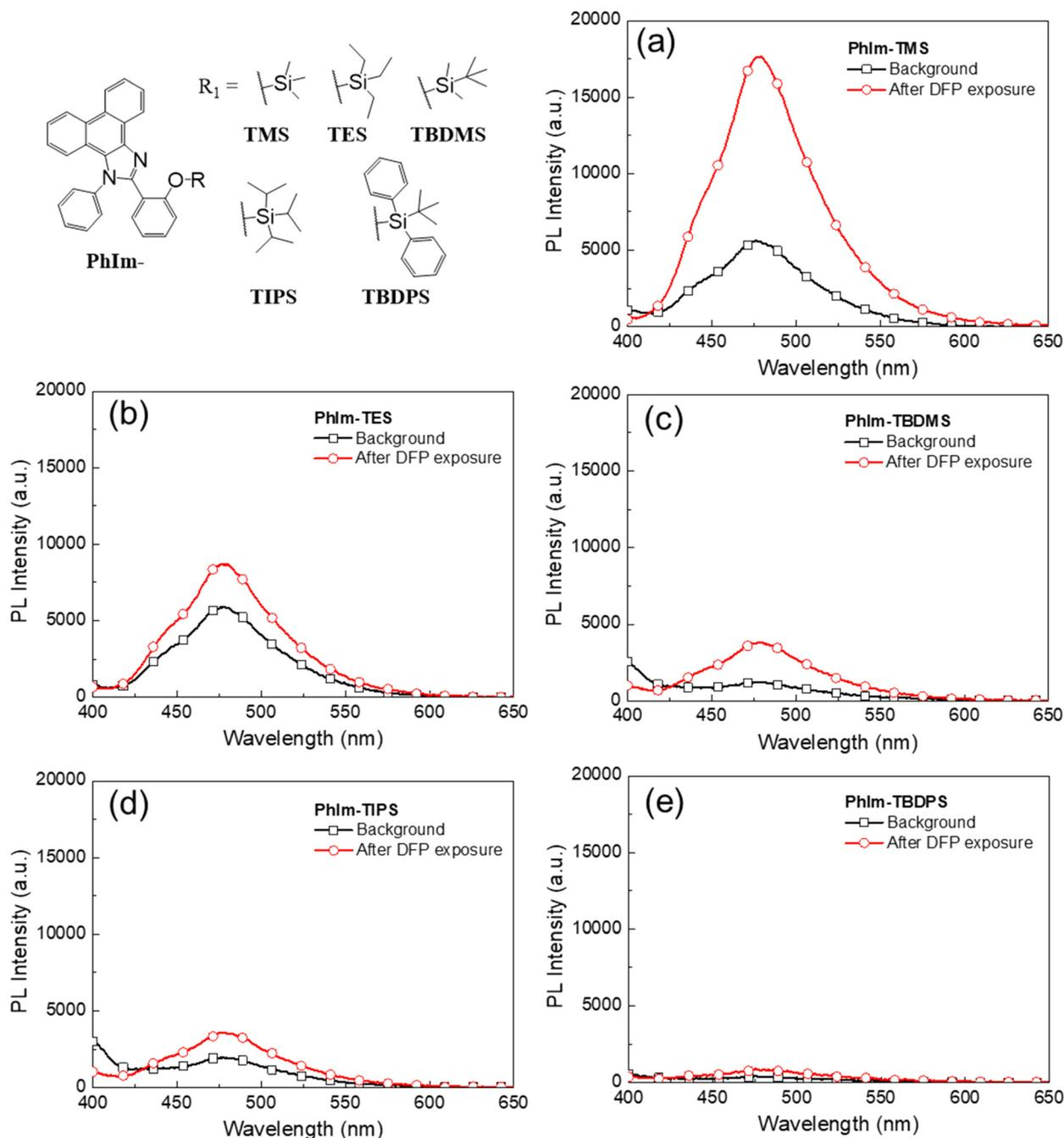
**Fig. 4** PL spectra of PhIm- (a) TMS, (b) TES, (c) TBDMS, (d) TIPS, and (e) TBDPS silyl ethers after 2 hours under ambient conditions (background) and then exposure to 95% DFP headspace vapours. Saturated DFP vapours (3 mL) were injected at  $20 \text{ mL min}^{-1}$  into a nitrogen flow ( $200 \text{ mL min}^{-1}$ ) and the spectra were collected 10 seconds after completion of the injection. The films were excited at 365 nm using an LED light source.
