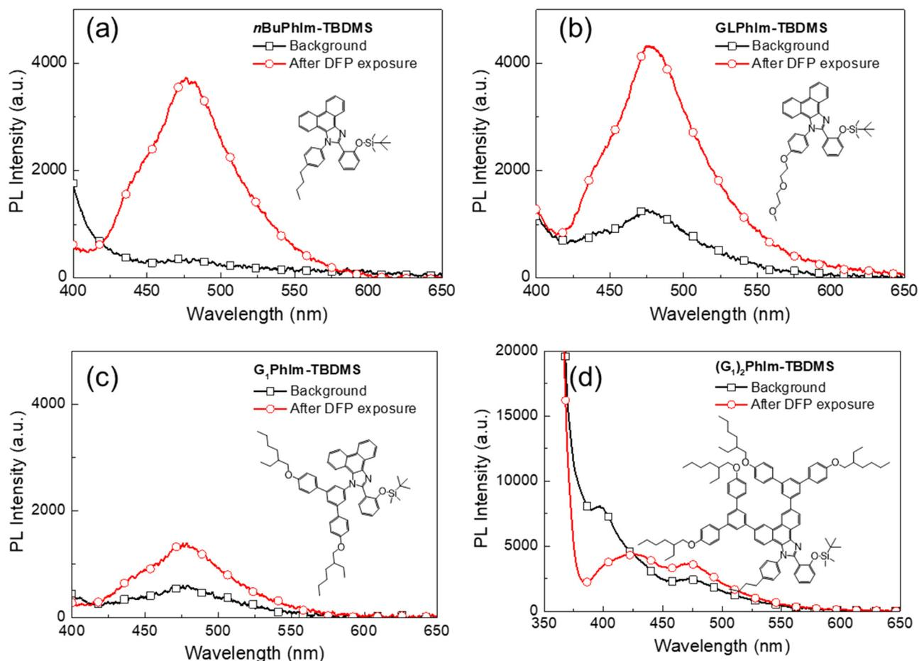
Fig. 6 PL spectra of (a) *n*-butyl, (b) glycol or (c and d) dendron-containing PhIm silyl ethers after 2 hours under ambient conditions (background) and then exposure to DFP of 95% purity. Saturated DFP vapours (3 mL) were injected at 20 mL min<sup>-1</sup> into a nitrogen gas flow (200 mL min<sup>-1</sup>). The films were excited at 365 nm using an LED light source.
