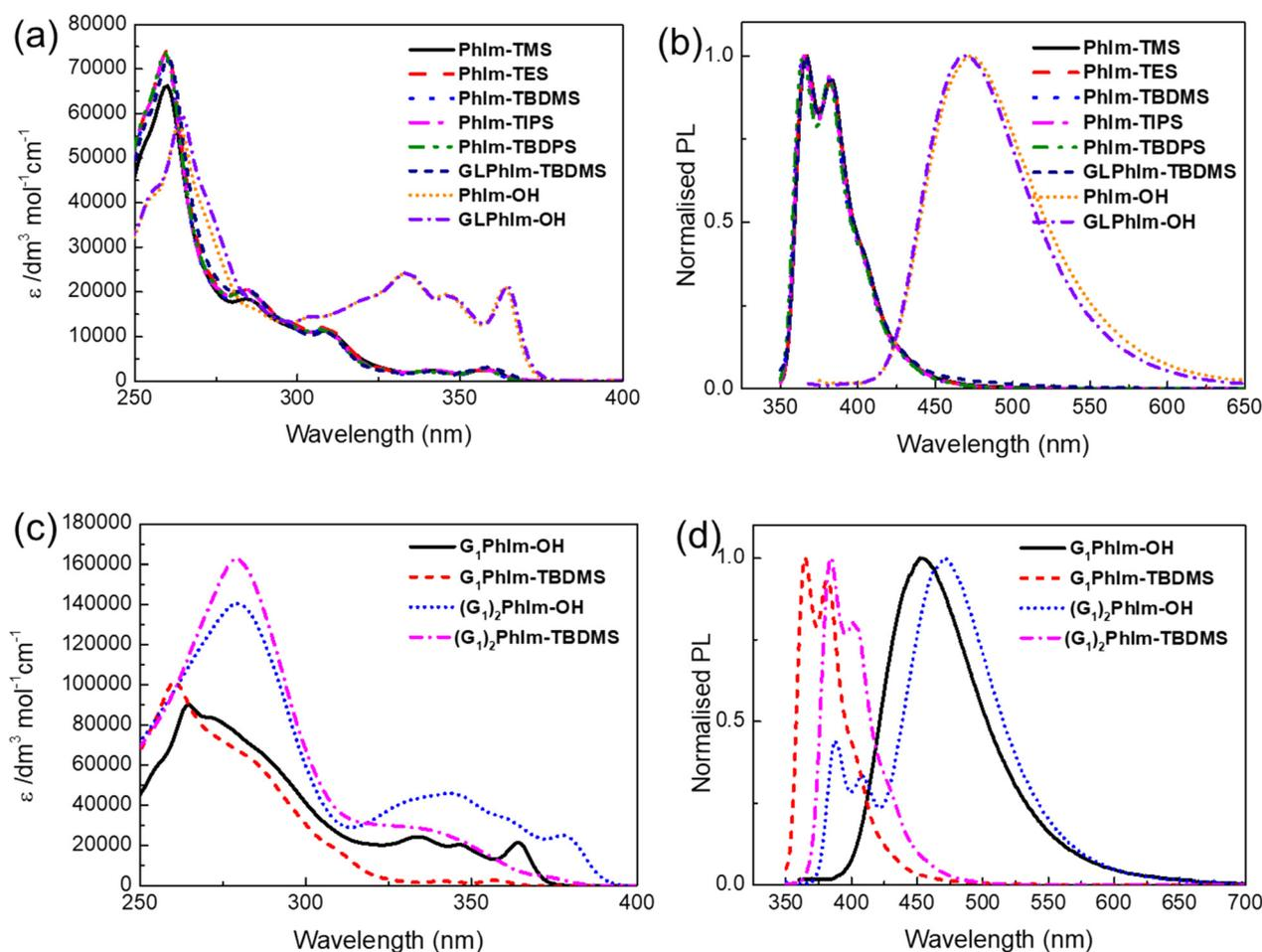
Fig. 3 Solution (dichloromethane) (a) UV-vis absorption and (b) PL spectra of **PhIm-OH**, **PhIm-Silyl ether**, **GLPhIm-OH** and **GLPhIm-TBDMS**, and (c) UV-vis absorption and (d) PL spectra of **G<sub>1</sub>PhIm-OH**, **G<sub>1</sub>PhIm-TBDMS**, **(G<sub>1</sub>)<sub>2</sub>PhIm-OH** and **(G<sub>1</sub>)<sub>2</sub>PhIm-TBDMS**.
