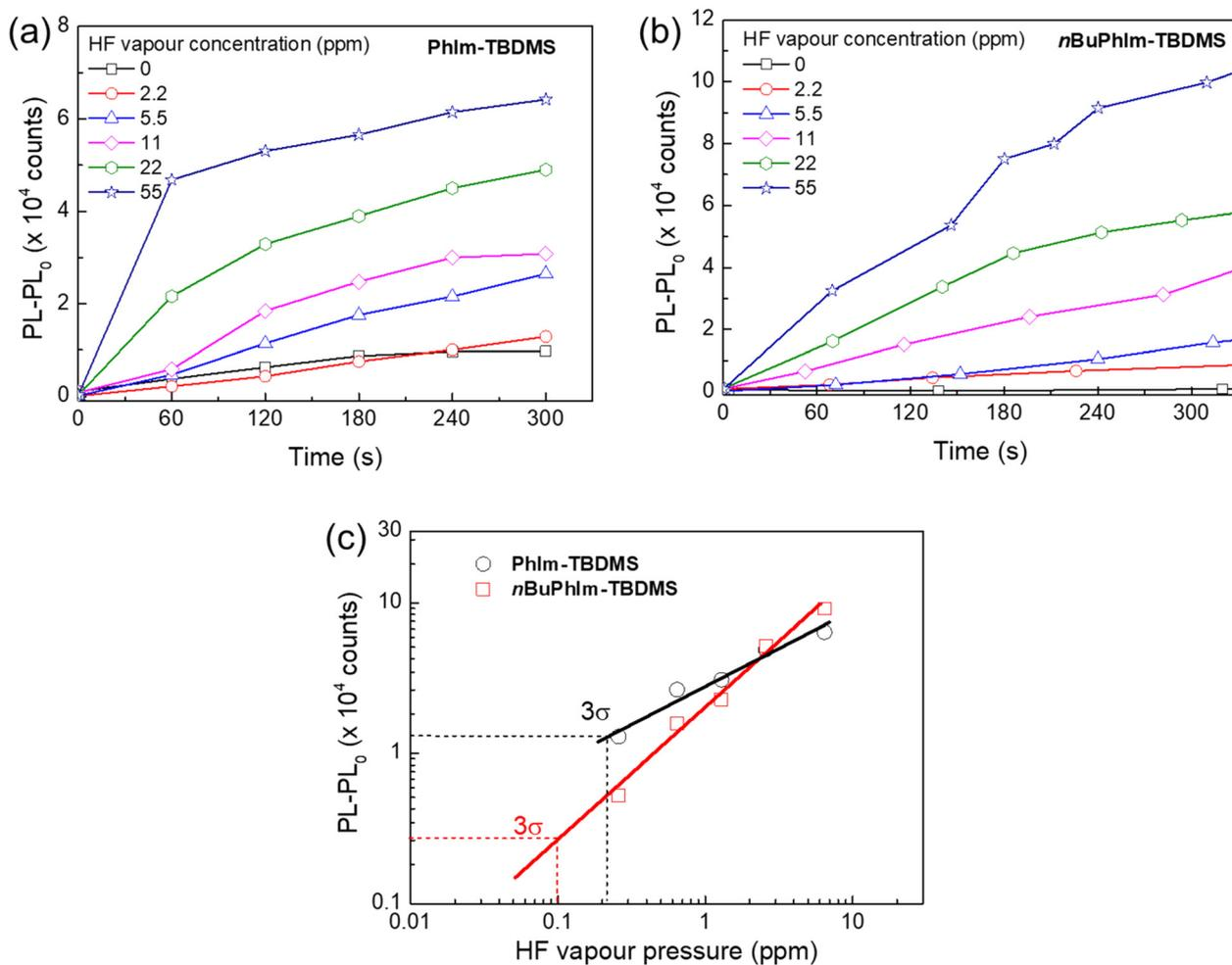
**Fig. 8** PL responses of (a) PhIm and (b) *n*BuPhIm-based sensing materials against HF vapour concentration, and (c) estimation of the LoD using three times the standard deviation ( $3\sigma$ ) of the change in PL intensity in air. Saturated DFP vapour was continuously injected at a rate of 0–5 mL  $\text{min}^{-1}$  into a nitrogen flow (200 mL  $\text{min}^{-1}$ ). The DFP purity was 99%. The films were excited at 365 nm using an LED light source.
