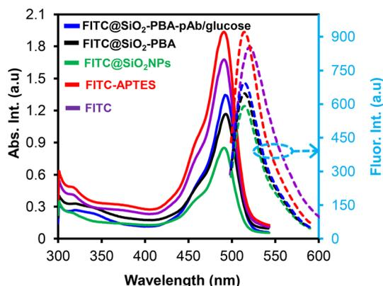
Fig. 3 Ground state absorption (solid lines) and fluorescence emission (dotted lines) spectra of FITC (1), FITC-APTES (3), FITC@SiO<sub>2</sub>NPs, FITC@SiO<sub>2</sub>-PBANPs, and FITC@SiO<sub>2</sub>-PBA-pAb (the colours show reference to the materials).
