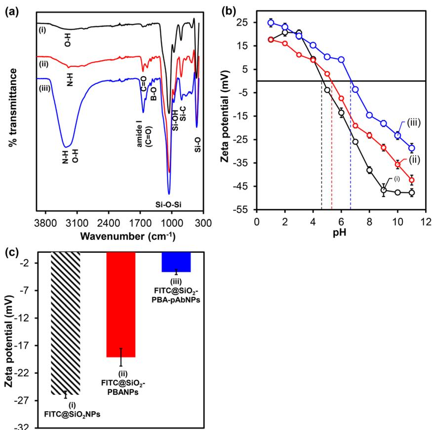
**Fig. 1** (a) FTIR spectra, (b) zeta potential (mV) vs. pH, and (c) bar graph of zeta-potential at pH (7.0) of (i) FITC@SiO<sub>2</sub>NPs, (ii) FITC@SiO<sub>2</sub>-PBANPs, and (iii) FITC@SiO<sub>2</sub>-PBA-pAb. The data in (b) and (c) were measured in triplicates ( $n = 3$ ).
