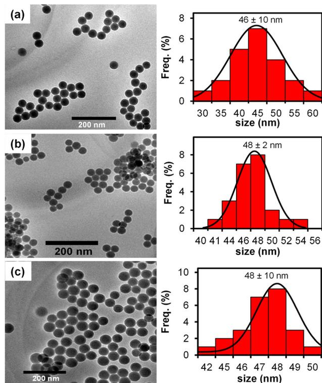
Fig. 2 TEM micrographs and corresponding histograms of 6% (a) FITC@SiO<sub>2</sub>NPs, (b) FITC@SiO<sub>2</sub>-PBANPs, and (c) FITC@SiO<sub>2</sub>-PBA-pAb/glucose.
