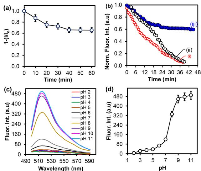
**Fig. 4** Fluorescence intensity over time for (a) dye-leakage studies of FITC@SiO<sub>2</sub>NPs, (b) photostability studies of (i) FITC (1), (ii) FITC-APTES (2), and (iii) FITC@SiO<sub>2</sub>NPs, (c) fluorescence spectra, and (d) corresponding fluorescence intensity of FITC@SiO<sub>2</sub>NPs at varied pH (2.0–11.0) in PBS (10 mM).
