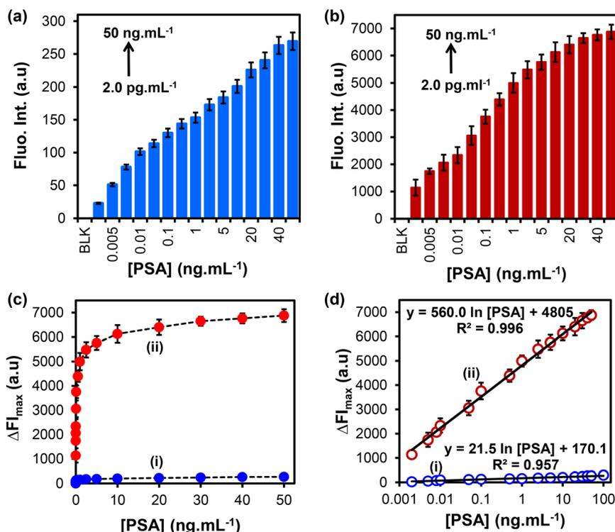
**Fig. 5** Fluorescence emission of the FITC@SiO<sub>2</sub>-PBA-pAb/glucose nanobioconjugates at increasing PSA concentrations from (2.0 pg mL<sup>-1</sup>–100 ng mL<sup>-1</sup>) (a) before and (b) after NaOH dissolution. (c) Dose-response curves and (d) calibration curve of relative fluorescence intensity ( $\Delta FI_{max}$ ) vs. [PSA] (i) before and (ii) after dissolution with NaOH (10 mM) ( $n = 3$ ).
