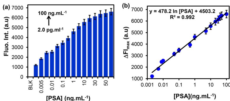
Fig. 6 (a) Fluorescence emissions for different concentrations of PSA (2.0 pg mL<sup>-1</sup>–100 ng mL<sup>-1</sup>), (b) calibration curve of relative fluorescence intensity ( $\Delta FI$ ) against [PSA] in the spiked new-born calf serum (2.0–100 ng mL<sup>-1</sup>) ( $n = 3$ ).
