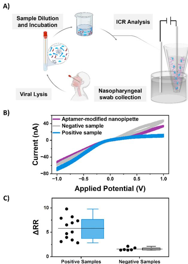
**Fig. 4** (A) An illustration of the sample collection and preparation utilized for ICR-based detection. (B) Sample *I-V* curves and (C) a bar plot of the average change in the rectification ratio of aptamer-modified nanopipettes (purple) incubated in positive (blue) and negative (grey) SARS-CoV-2 patient samples. Each data point represents a measurement from a unique sample.
