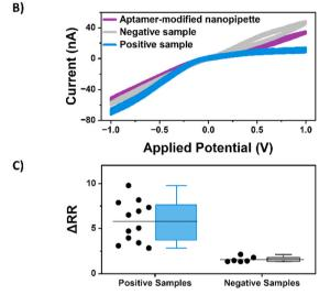
Fig. 4 (A) An illustration of the sample collection and preparation utilized for ICR-based detection. (B) Sample I-V curves and (C) a bar plot of the average change in the rectification ratio of aptamermodified nanopipettes (purple) incubated in positive (blue) and negative (grey) SARS-CoV-2 patient samples. Each data point represents a measurement from a unique sample.
