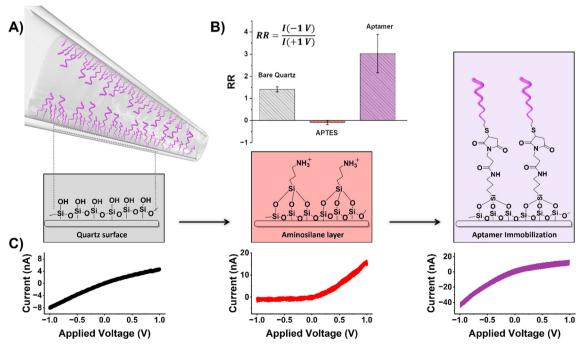
Fig. 1 (A) The stepwise functionalization of a quartz nanopipette with an aptamer-selective for the S1 domain of SARS-CoV-2. (B) The average rectification ratio and (C) a sample I-V curve for each modification step in 0.01 M KCl. Error bars represent the standard error from a minimum of six measurements, each with a different functionalized nanopipette.
