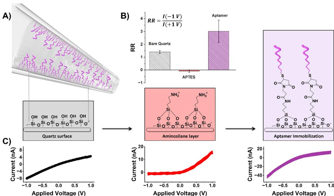
Fig. 1 (A) The stepwise functionalization of a quartz nanopipette with an aptamer-selective for the S1 domain of SARS-CoV-2. (B) The average rectification ratio and (C) a sample  $I$ - $V$  curve for each modification step in 0.01 M KCl. Error bars represent the standard error from a minimum of six measurements, each with a different functionalized nanopipette.
