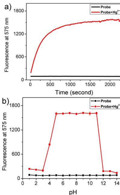
**Fig. 3** a) Time-dependent fluorescence change (at 575 nm) of Rh-Ip-Hy (5  $\mu\text{M}$ ) with the addition of  $\text{Hg}^{2+}$  (10 equiv.) in the PBS buffer solution (10 mM, EtOH/ $\text{H}_2\text{O}$  = 1/4, pH of 7.4). b) Profile of pH dependence of the fluorescence intensity of the probe (5  $\mu\text{M}$ ) at 575 nm in the absence and presence of  $\text{Hg}^{2+}$  (10 equiv.) in the PBS buffer solution (10 mM, EtOH/ $\text{H}_2\text{O}$  = 1/4).
