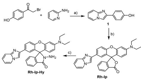
**Scheme 2** Synthesis routes of **Rh-Ip-Hy**. Reagents and conditions: a)  $\text{Na}_2\text{CO}_3$ , EtOH, reflux for 20 h; b) 2-(4-(*N,N*-diethylamino)-2-hydroxybenzoyl)benzoic acid, TFA/ $\text{MeSO}_3\text{H}$  (v/v, 1/1), 80 °C for 24 h; c) hydrazine hydrate, EtOH, 100 °C for 4 h.
