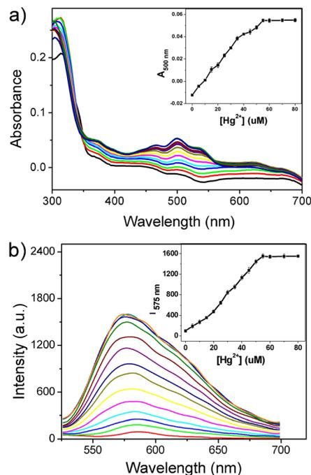
**Fig. 1** a) UV-vis and b) fluorescence spectra of **Rh-Ip-Hy** (5  $\mu\text{M}$ ) after adding increasing amounts of  $\text{Hg}^{2+}$  in the PBS buffer (10 mM, EtOH/ $\text{H}_2\text{O} = 1/4$ , pH of 7.4). Insets: the corresponding intensity changes of the probe as a function of  $\text{Hg}^{2+}$  concentration.
