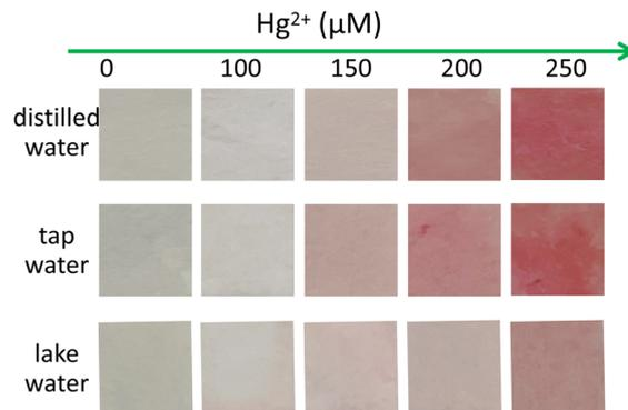
Fig. 6 Visualization of  $\text{Hg}^{2+}$  using the test strips prepared with **Rh-Ip-Hy** in distilled water, tap water and lake water, respectively.
