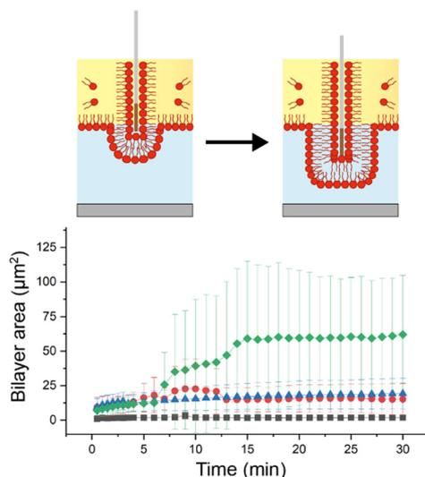
**Fig. 4** Control of bilayer area by lowering the measuring electrode to different positions through the oil-water interface. Data points correspond to translation distances of 1.5 mm ( $n = 3$ , squares), 2.0 mm ( $n = 6$ , circles), 2.5 mm ( $n = 5$ , triangles) and 3.0 mm ( $n = 4$ , diamonds). The data shows that the area of the bilayer increases with translation distance. Illustrations do not show the ground electrode.
