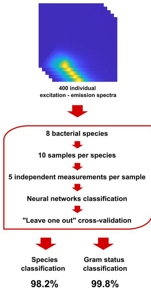
**Fig. 4** Workflow of the classification experiment using 8 representative bacterial species: the main dataset of 400 excitation-emission spectra was used to train a neural network classifier, and its accuracy was determined for classification at the Gram status and species levels.
