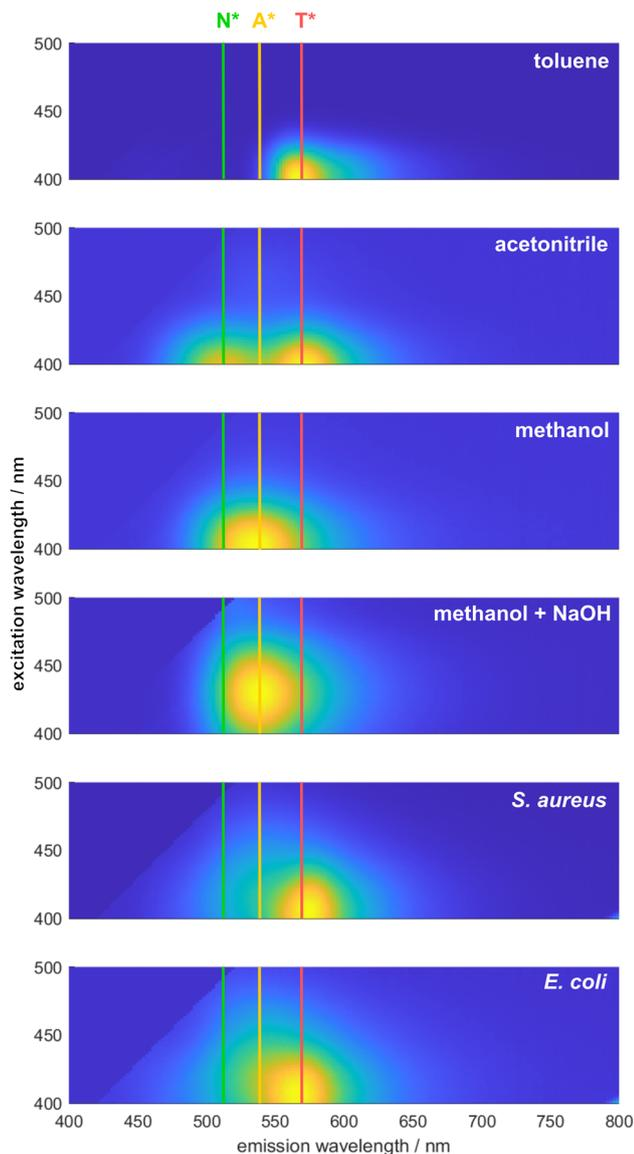
**Fig. 2** Excitation–emission spectra of DMAF in non-polar (toluene), polar aprotic (acetonitrile), polar protic (methanol) and basic (methanol + NaOH) environments, as well as in PBS with addition of *S. aureus* and *E. coli*. The lines serve as guides to the eye for the positions of emission maxima of the normal ( $N^*$ ), anionic/H-bonded ( $A^*$ ) and phototautomeric ( $T^*$ ) forms of DMAF.
