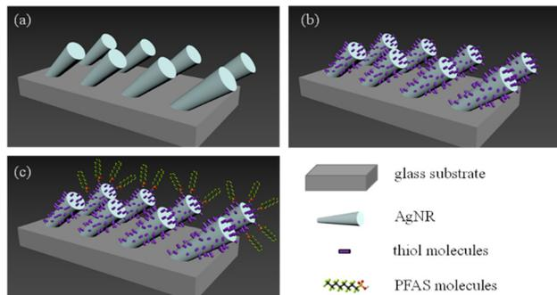
**Fig. 1** (a) Ag nanorods on a glass substrate. (b) A self-assembled monolayer of thiol molecules coats the nanorods. (c) The charged PFAS molecules are electrostatically attracted to the thiol molecule monolayer.
