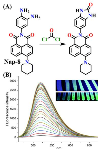
Fig. 6 (A) Structure of sensor Nap-8 and its products upon reaction with phosgene. (B) The gradual increase in the emission intensity of Nap-8 upon increasing the concentration of phosgene in the  $\text{CH}_2\text{Cl}_2$  (inset: visual color changes in solution and gas phase after exposure to phosgene at different concentrations). Reproduced with permission from ref. 57. Copyright 2023, Elsevier.
