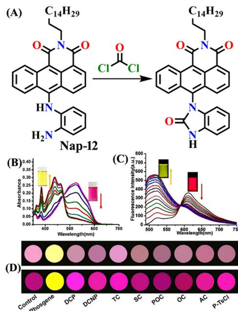
**Fig. 10** (A) Structure of sensor Nap-12 and its carboximide product upon reaction with phosgene. The observed changes in (B) UV-visible absorption and (C) fluorescence emission spectra of Nap-12 after the gradual addition of the phosgene (inset: photographs of visual color changes). (D) TLC plates for color and fluorescence color changes for Nap-12 in the presence of different analytes. Reproduced with permission from ref. 61. Copyright 2019, Elsevier.
