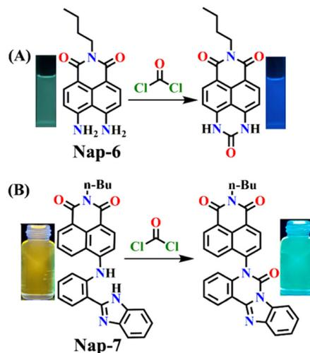
**Fig. 5** (A) Structure of sensor Nap-6 and its products upon reaction with phosgene and their corresponding colorimetric images. (B) Structure of sensor Nap-7 and its products upon reaction with phosgene and their corresponding colorimetric images. Reproduced with permission from ref. 54 and 56. Copyright 2019, Wiley; Copyright 2022, Elsevier.
