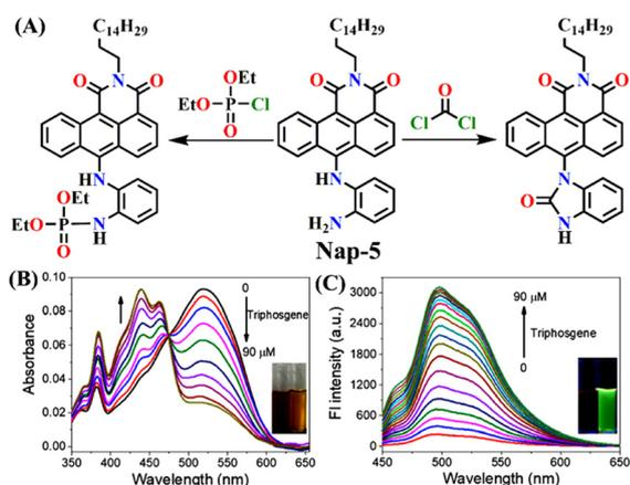
**Fig. 4** (A) Structure of sensor Nap-5 and its products upon reaction with phosgene and chlorophosphate. (B) Changes in UV-visible absorption and (C) fluorescence emission spectra of Nap-5 upon the gradual addition of triphosgene in  $\text{CH}_2\text{Cl}_2$  solution (inset: visual color changes before and after the addition of triphosgene seen under UV light). Reproduced with permission from ref. 8. Copyright 2019, American Chemical Society.
