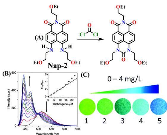
**Fig. 2** (A) Structure of Nap-2 and its product upon reaction with phosgene. (B) Ratiometric fluorescence responses were observed for Nap-2 upon the gradual increase in triphosgene solution (inset: a plot of the fluorescence intensity ratio and the concentration of triphosgene). (C) Photographs of Nap-2 coated test papers after exposure to triphosgene at different concentrations. Reproduced with permission from ref. 31. Copyright 2017, the Royal Society of Chemistry.
