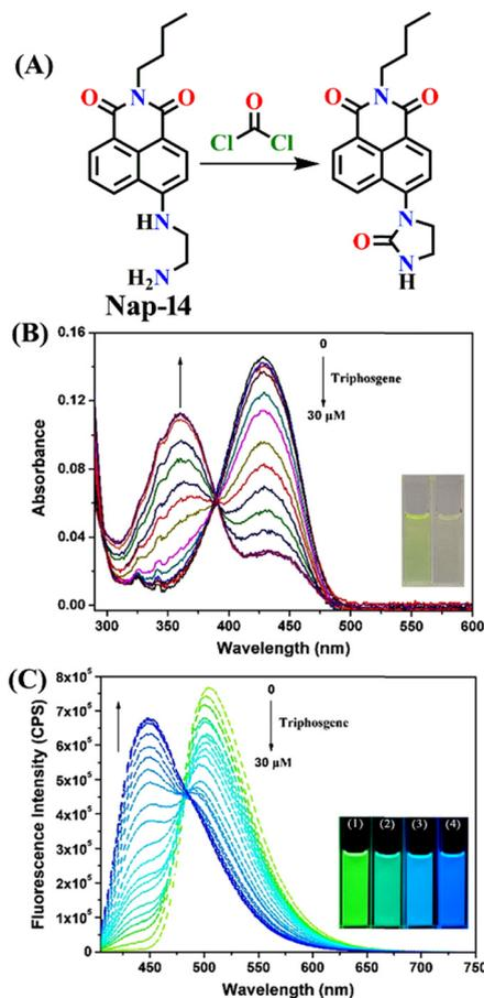
**Fig. 12** (A) Structure of sensor Nap-14 and its product formed after reaction with phosgene. Relative changes in (B) UV-visible and (C) fluorescence emission spectra of Nap-14 upon increasing the triphosgene concentrations (inset: corresponding colorimetric photographs). Reproduced with permission from ref. 62. Copyright 2022, Elsevier.
