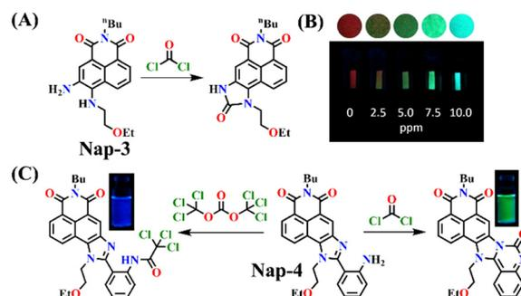
**Fig. 3** (A) Structure of Nap-3 and its product upon reaction with phosgene. (B) Fluorescence images of Nap-3-coated test paper after exposure to diphosgene vapors at different concentrations. (C) The distinct reaction of Nap-4 with phosgene and triphosgene yielded green and blue-emitting products, respectively (inset: colorimetric photo). Reproduced with permission from ref. 30 and 53. Copyright 2018, Wiley; 2019, American Chemical Society.
