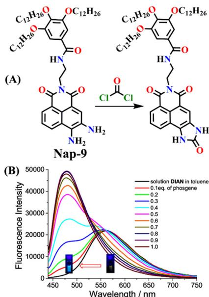
**Fig. 7** (A) Structure of sensor Nap-9 and its products upon reaction with phosgene and thionyl chloride. (B) The observed changes in fluorescence emission intensity for Nap-9 after a gradual increase in phosgene concentration (inset: colorimetric photographs). Reproduced with permission from ref. 37. Copyright 2023, American Chemical Society.
