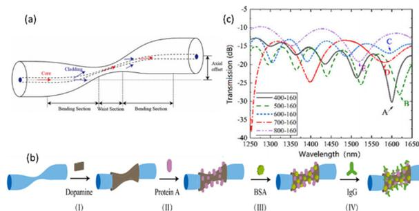
Fig. 16 (a) Schematic of the STF sensor, (b) protein A-IgG binding reaction, and (c) transmission spectra of STF.
