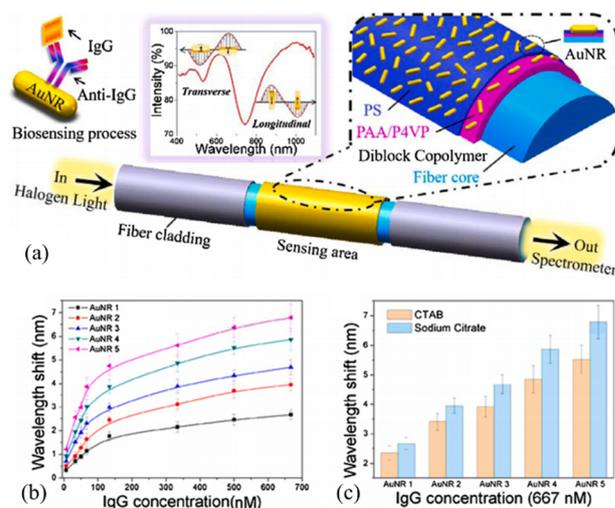
**Fig. 6** (a) Schematic diagram of the AuNR-coated LSPR optical fiber biosensor; (b) calibration curve of the LSPR peak wavelength change for different concentrations of human IgG; (c) peak wavelength shift at a human IgG concentration of 667 nM.
