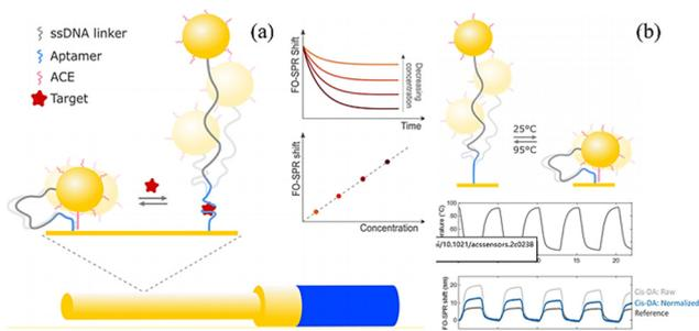
**Fig. 7** (a) Schematic representation of the proposed bioassay, where *cis*-DAs are implemented on a FO-SPR sensor; (b) schematic representation of the switching between the “distal” and “proximal” state of *cis*-DA, induced by temperature cycles between 95 and 25 °C.
