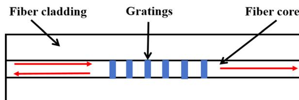
Fig. 24 Basic structure of the fiber Bragg grating.
