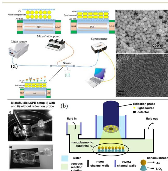
Fig. 22 Interactions of biological molecules in the immune system based on the optical fiber SPR sensor: (a) Xia *et al.*<sup>104</sup> and (b) J. Roether *et al.*<sup>105</sup>
