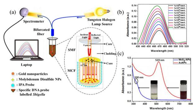
**Fig. 10** (a) Experimental setup for the detection of Shigella bacteria and (b) UV-vis spectra of the AuNPs, and (c) MoS<sub>2</sub>-NPs solutions and corresponding photographs.
