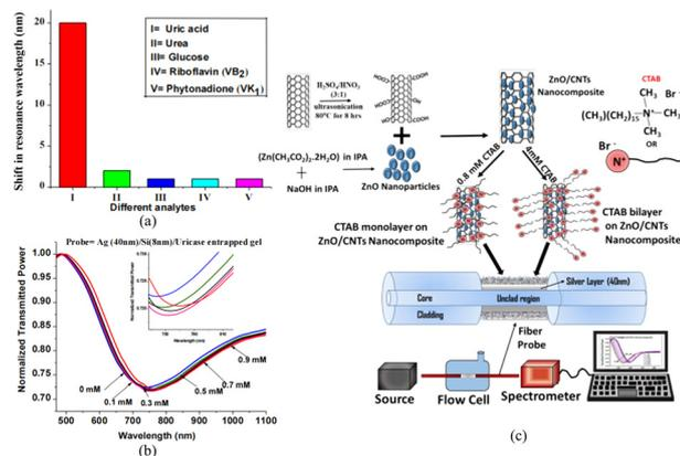
**Fig. 4** (a) Shifts in the resonance wavelength for different analytes; (b) experimental SPR spectra for the optical fiber SPR probe for uric acid; (c) schematic showing the synthesis of functionalized CNTs and ZnO nanoparticles, attachment of ZnO nanoparticles to CNT walls, CTAB functionalization of the ZnO/CNTs nanocomposite for two concentrations, fiber probe and experimental set-up.
