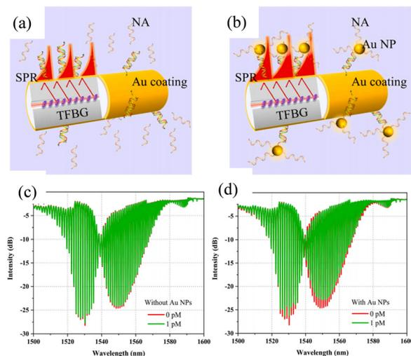
**Fig. 31** Enhancement of sensitivity to NA of a TFBG-SPR sensor by using gold nanoparticles bonded onto the target NA chains. (a and b) Schematic representations of the sensing scheme (a) without and (b) with gold nanoparticles. (c and d) Transmission spectra of the sensor (c) without and (d) with gold nanoparticles.
