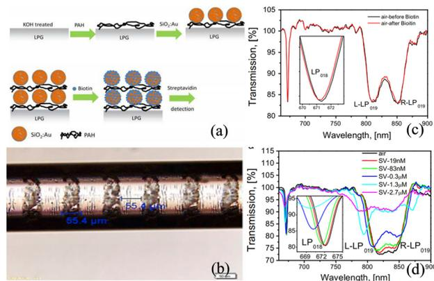
**Fig. 32** (a) Schematic illustration of layer-by-layer deposition of a (PAH/SiO<sub>2</sub>: Au)<sub>2</sub> film on the optical fiber LPG; (b) optical image of LPG; (c) transmission spectra of LPG coated with (PAH/SiO<sub>2</sub>(300 nm): Au)<sub>3</sub> exposed to (c) biotin and (d) streptavidin with different concentrations.
