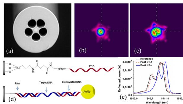
**Fig. 26** (a) Scanning electron micrograph of a microstructured optical fiber (MOF); (b) basic profile and (c) first-order beam profile; (d) schematic showing the linkage of the peptide nucleic acid (PNA) probe to the fiber internal surface and sandwich-like system used for DNA detection; (e) spectra after hybridization with 100 nM full-match DNA solution and gold nanoparticles.<sup>126</sup>
