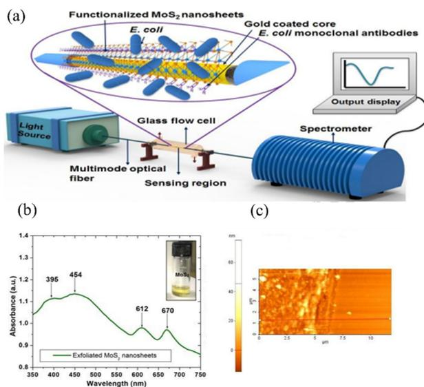
**Fig. 5** (a) Schematic of the experimental setup of the optical fiber SPR immunosensor for the detection of *E. coli*; (b) UV-vis absorption spectra of exfoliated MoS<sub>2</sub> nanosheets; (c) 2D contact mode AFM image of the MoS<sub>2</sub> nanosheets and the line scan.
