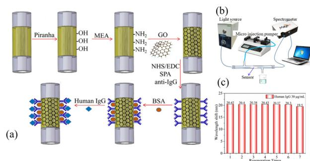
**Fig. 9** (a) Graphene oxide and SPA modification of the IgG immunoassay, (b) schematic of the experimental setup of the goat anti-human IgG sensor, and (c) regeneration performance of the Au/GO-SPA immunosensor.
