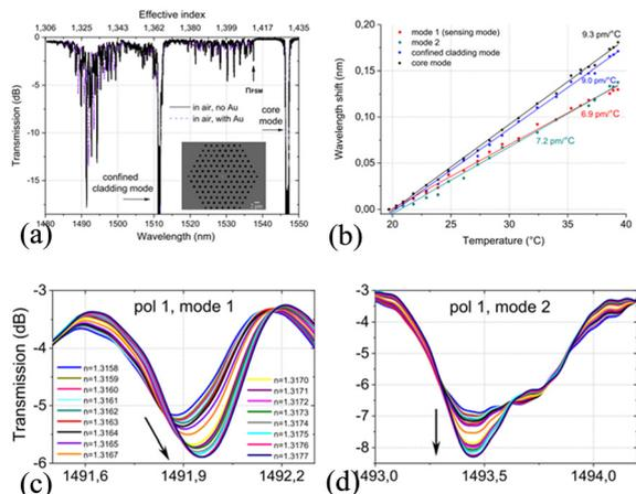
**Fig. 27** (a) Transmission spectra of FBG in PCF (micrographs of cross-sections shown); (b) resonance wavelengths for the selected modes showing different dependence on the temperature variations in water; (c and d) transmission spectra of modes 1 and 2 after immersion of the gold-coated PCF gratings in solutions with 17 refractive indexes; modes showing the largest shifts in wavelength and amplitude in the SPR-excited state.<sup>128</sup>
