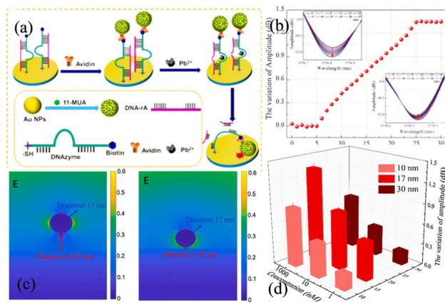
**Fig. 30** (a) Schematic showing lead detection by the TFBG-SPR sensing system; (b) amplitude responses of the TFBG-SPR sensing cladding modes; (c) electric field distributions of the gold nanoparticles on the Au film with gap distances of 16.02 nm and 1.52 nm; (d) effects of gold nanoparticles with different sizes on the signals.<sup>139</sup>
