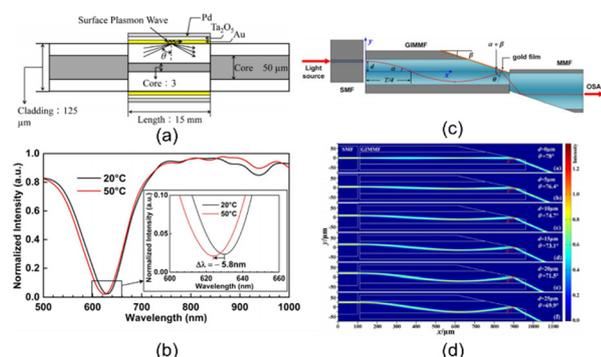
**Fig. 8** (a) Micro-displacement fiber sensor and (b) micro-displacement sensor; (c) dependence of the wavelength and resonance intensity at different temperatures and (d) beam paths when the offset value  $d$  increases from 0 to 25  $\mu\text{m}$  by simulation.
