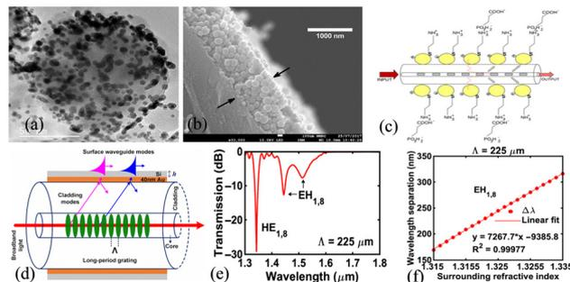
**Fig. 33** (a) TEM image of SiNPs with a gold shell,<sup>149</sup> (b) cross-sectional image of the optical fiber with three layers of PAH/SiNPs and gold shell; (c) schematic drawing of the LPFG-AuNP-Cys fiber sensor,<sup>150</sup> (d) LPFG coated with gold-silicon films; (e) transmission spectrum for the 225  $\mu\text{m}$  grating period; (f) wavelength variation and sensitivity of the EH<sub>1,8</sub> modes.<sup>151</sup>
