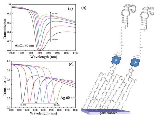
**Fig. 11** (a) Transmission spectra of the SPR sensor with different Al<sub>2</sub>O<sub>3</sub> thicknesses, (b) functionalization process,<sup>66</sup> and (c) SPR transmission spectra for different concentrations of thrombin (1–80 nM).
