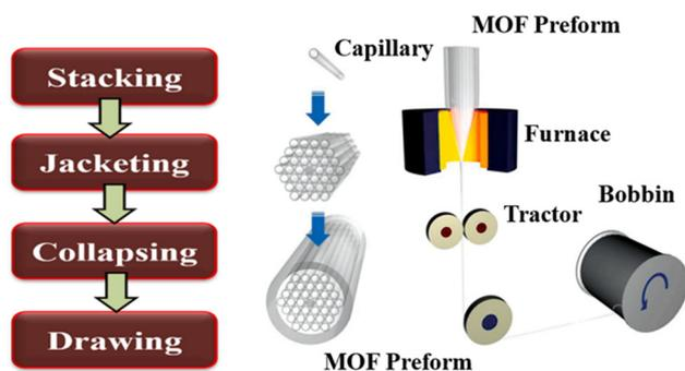
Fig. 19 Fabrication of MOFs by the stack-and-draw method.
