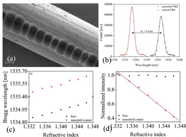
**Fig. 25** (a) SEM image of etched FBG with a nanoshell coating and an increased particle density in the microstructured fiber grating area; (b) reflecting spectra of the unetched and etched FBG; SRI-dependent sensing response of the bare and nanoshell coated fiber tip; (c) Bragg wavelength and (d) amplitude.<sup>123</sup>
