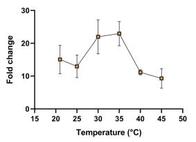
Fig. 2 Influence of assay temperature while using short probe in flow-based miR-122 hybridisation system. EIS signals (fold change) from electrodes functionalised with 6  $\mu$ M P-S3<sub>10</sub> after 60 min incubation with 10 nM miR-122 at 100  $\mu$ L min<sup>-1</sup> flow rate and at room temperature (21 °C) to varying hybridisation temperatures (21–45 °C). All data represent the mean  $\pm$  SD; n=3.
