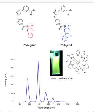
Fig. 23 Structures of ligands Phe & Trp, and the delayed luminescence spectra of [Tb(Phe)<sub>3</sub>]<sup>3+</sup> recorded in MeCN. Inset: Picture of complex solution under illumination via UV lamp (adapted from ref. 205 with permission from Royal Society of Chemistry, copyright 2023).205
