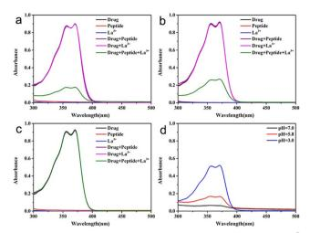
**Fig. 31** Drug-loading and release of camptothecin *via* DDColDD-La<sup>3+</sup>. Absorbance spectra at (a) pH = 7.0, (b) pH = 5.8, (c) pH = 3.0. Absorbance spectra of camptothecin release within the supernatant after 24 h (d) (reprinted from ref. 241 with permission from American Chemical Society, copyright 2019).  $^{241}$
