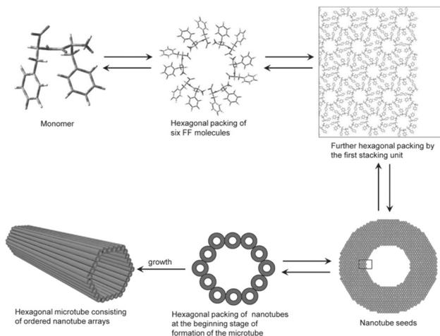
**Fig. 4** Schematic illustration of the formation of hexagonal peptide microtubes via L-Phe-L-Phe molecules (reprinted from ref. 28 with permission from John Wiley and Sons, copyright 2011).<sup>28</sup>
