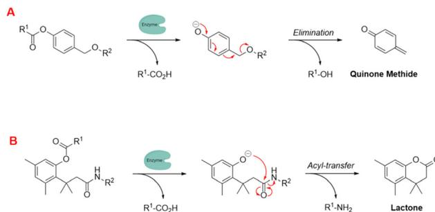
**Fig. 18** Examples of self-immolative linker strategies – mechanism(s) of activation, (A) elimination and (B) acyl-transfer (adapted from ref. 164 with permission from American Chemical Society, copyright 2018).<sup>164</sup>
