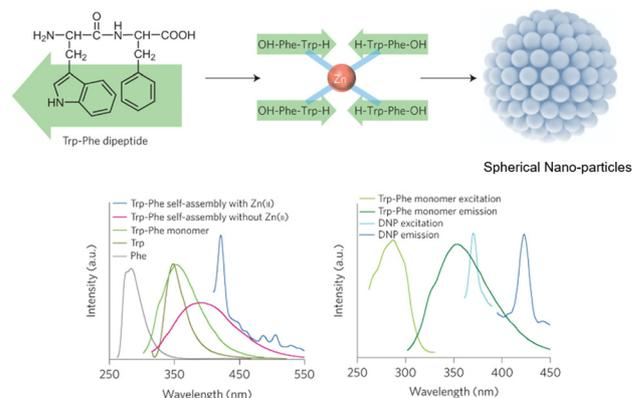
**Fig. 28** Design strategy for fluorescent nanoparticles *via* L-Trp-L-Phe self-assembly. (Bottom left) Various fluorescent emission spectra. (Bottom right) Fluorescent excitation and emission spectra of dipeptide monomers vs. self-assembled nanoparticles.<sup>235</sup>
