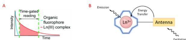
Fig. 22 Prolonged luminescence lifetime of the  $\text{Ln}^{3+}$  complex, in contrast to traditional organic fluorophores (A) (reprinted from ref. 198 with permission from Royal Society of Chemistry, copyright 2018).<sup>198</sup> Cartoon schematic of antenna excitation (B).
