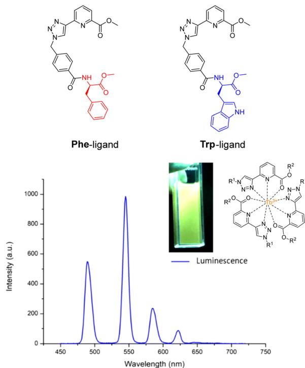
Fig. 23 Structures of ligands Phe & Trp, and the delayed luminescence spectra of  $[\text{Tb}(\text{Phe})_3]^{3+}$  recorded in MeCN. Inset: Picture of complex solution under illumination *via* UV lamp (adapted from ref. 205 with permission from Royal Society of Chemistry, copyright 2023).<sup>205</sup>
