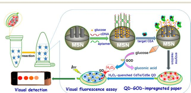
Fig. 17 Graphical illustration of the PAD for the visual fluorescence detection of CEA (reprinted from ref. 154 with permission from American Chemical Society, copyright 2017).<sup>154</sup>
