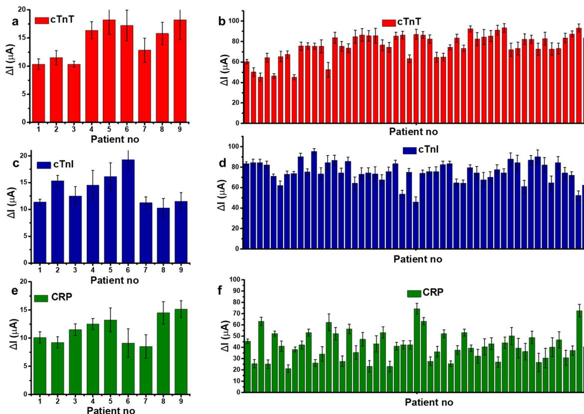
**Fig. 6** Histograms showing the change in oxidation current values ( $\Delta I$ ) of (a) cTnT, (c) cTnI, and (e) CRP sensors towards blood serum collected from control (negative) patients, (b) cTnT (d) cTnI, and (f) CRP sensors towards blood samples collected from AMI patients. Error bars show  $\pm$ SD for  $n = 3-5$  for different aptasensors. Measurements were performed under the same conditions as in Fig. 3.
