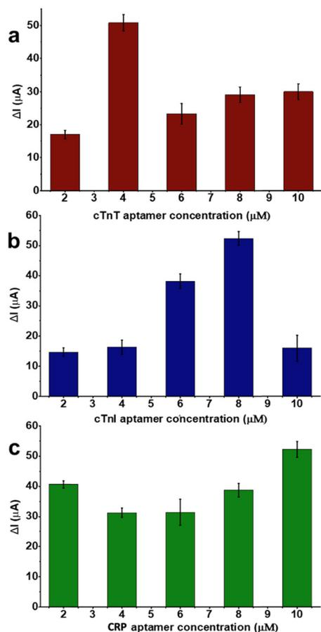
Fig. 3 Effect of aptamer concentrations of (a) cTnT, (b) cTnI, (c) CRP on the response signals. Measurements were performed at ambient conditions, in 0.1 M PBS and 0.1 M KCl containing 5.0 mM  $[\text{Fe}(\text{CN})_6]^{3-/4-}$ .
