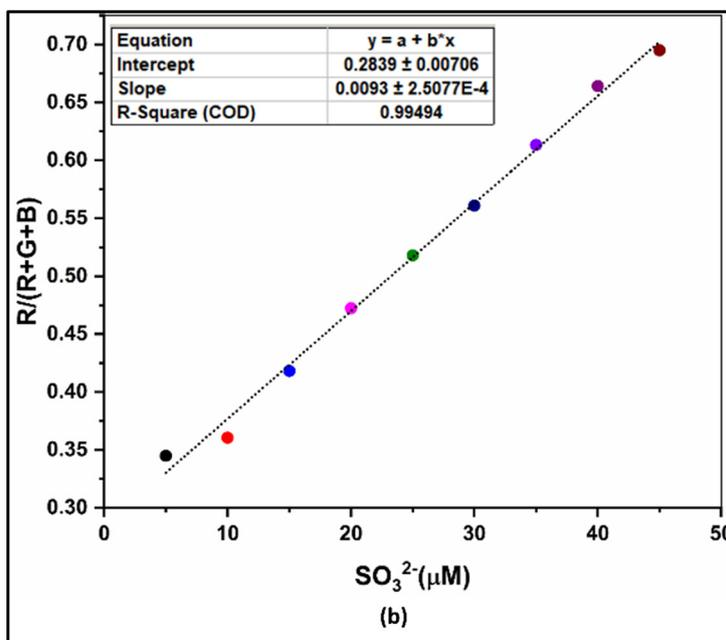
Fig. 11 (a) Integration of the BPPyz chemosensor with a smartphone and (b) the ratio of  $R/(R + G + B)$  versus  $\text{SO}_3^{2-}$  concentration in the range of 0 to 20.0  $\mu\text{M}$ .
