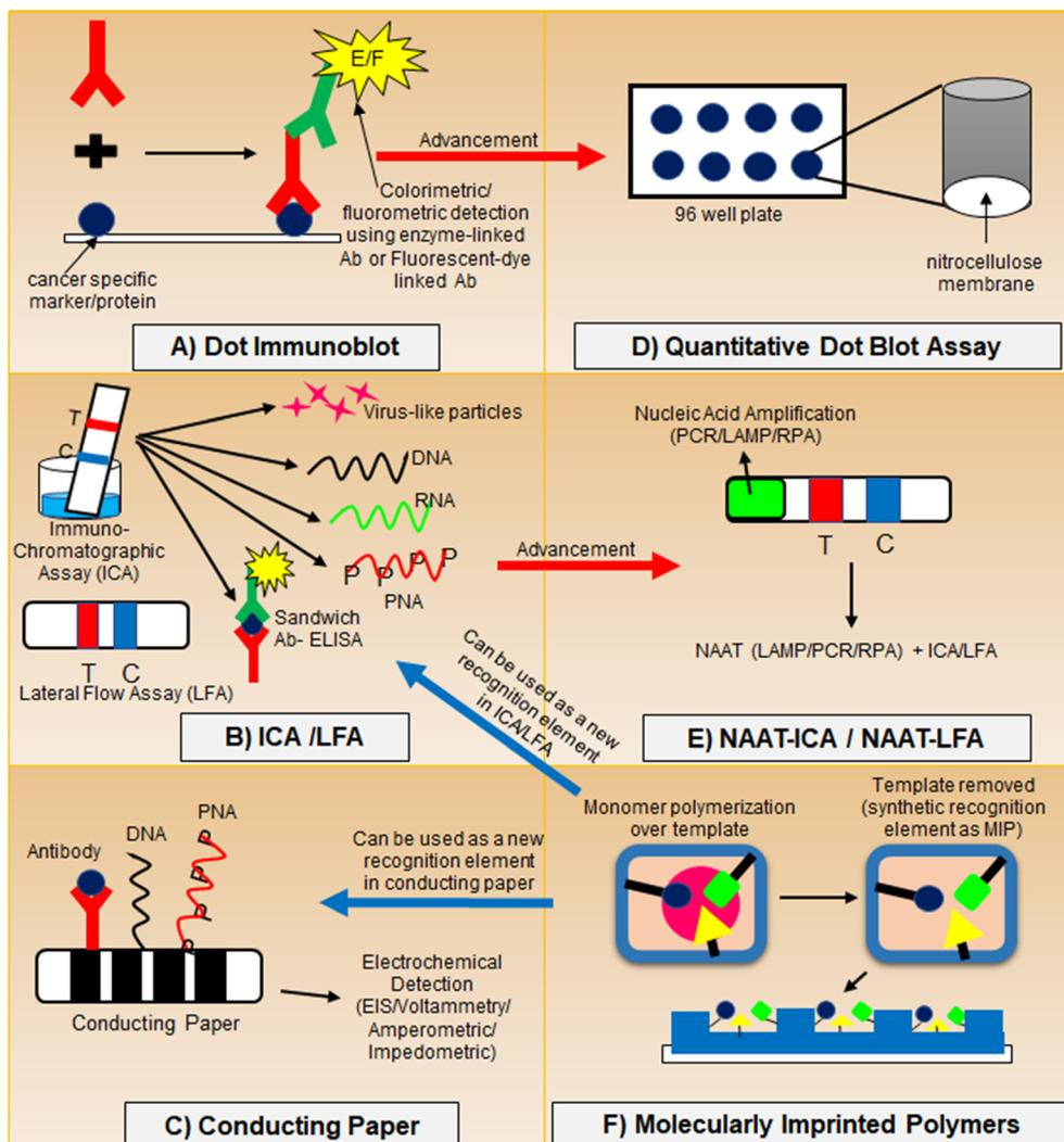
Fig. 2 Different mechanisms for the detection of analyte for paper-based diagnosis.
