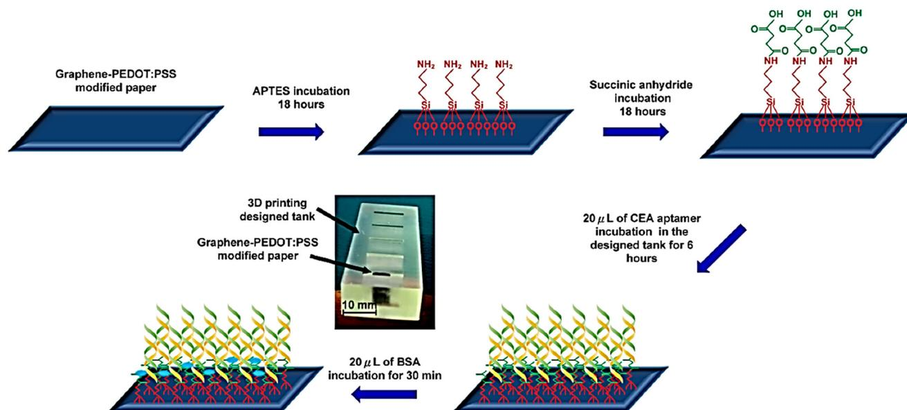
Fig. 5 Surface functionalization of conductive paper-based biosensor. Figure has been adapted with permission from Yen *et al.*, *Sensors*, 2020.<sup>84</sup>
