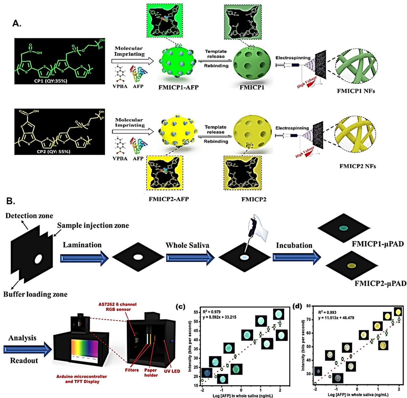
Fig. 4 A) Synthesis of molecularly imprinted nanofibres. B) Detection of AFP and CEA cancer biomarkers using MIP-coated  $\mu$ PAD device. Linear correlation between AFP concentration in whole saliva and the color intensity across the photodiode on C) FMICP1- $\mu$ PAD and D) FMICP2- $\mu$ PAD sensors. Figures A–D have been adapted with permission from Tawfik *et al.*, *Biosensors and Bioelectronics*, 2020.<sup>77</sup>
