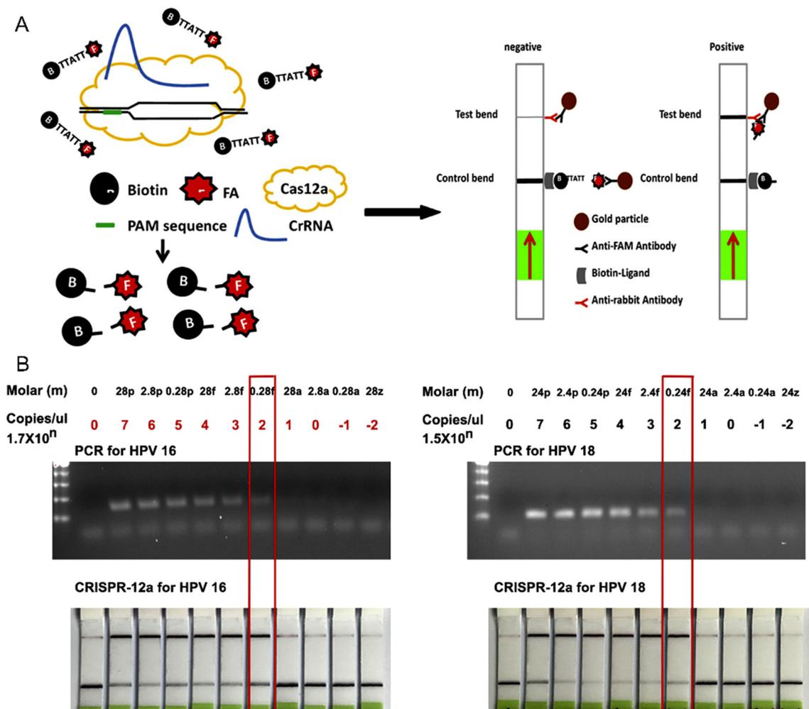
**Fig. 3** Schematic of the integrated CRISPR-Cas12a system with paper-based lateral flow assay for the detection of circulating nucleic acids (A), and comparative limit of detection of HPV 16 and 18 nucleic acids by PCR and CRISPR-Cas12a system with LFA in spiked samples (B). Figures A and B have been adapted with permission from Tsou *et al.*, Translation Oncology, 2019.<sup>70</sup>
