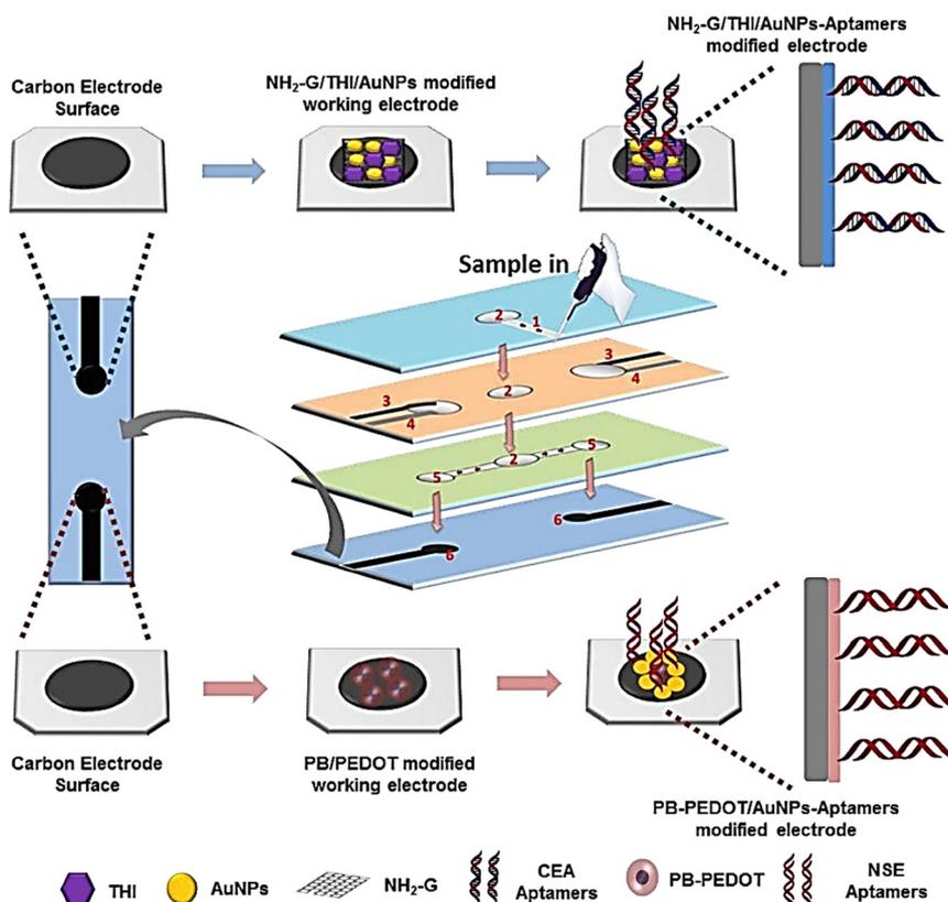
**Fig. 10** Paper-based electrochemical aptasensor. The working electrode was modified using amino functional graphene (NG)–thionin (THI)–gold nanoparticles (AuNPs) and Prussian blue (PB)–poly (3,4-ethylenedioxythiophene) (PEDOT)–AuNPs nanocomposites for the immobilization of the CEA and the NSE biomarkers as well as to promote electron transfer. Figure has been adapted with permission from Wang *et al.*, *Biosensors and Bioelectronics*, 2019.<sup>116</sup>
