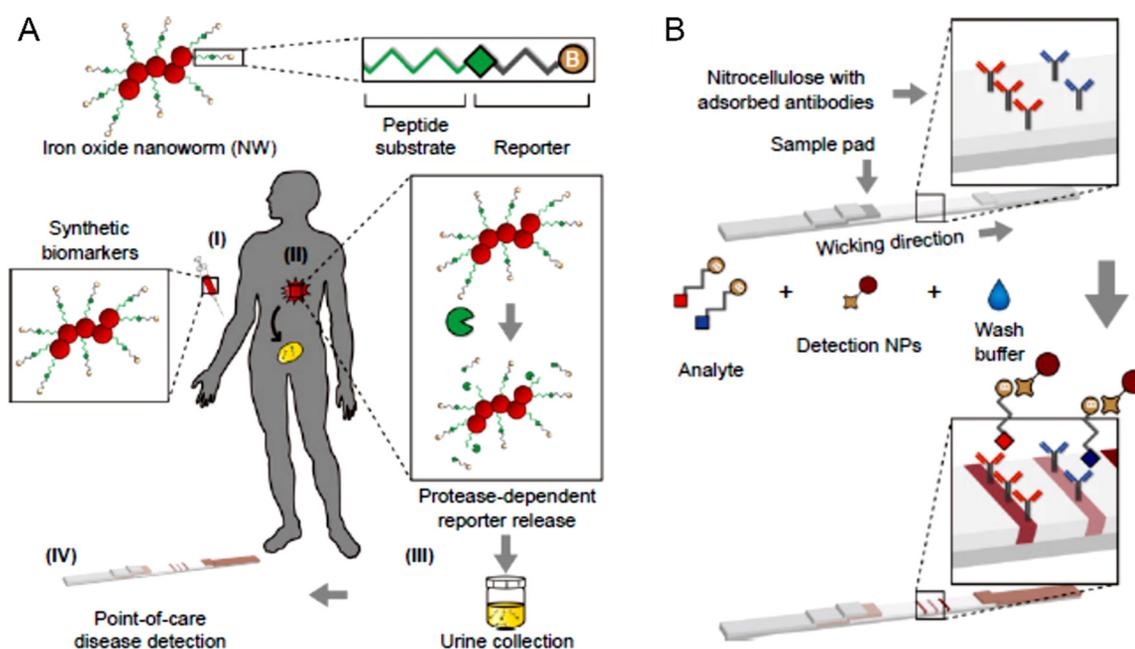
Fig. 12 Schematic of the synthetic urinary biomarker and steps involved in its *in vivo* processing to excrete detectable analyte in urine (A) and its subsequent paper-based detection (B). Figures A and B have been adapted with permission from Warren *et al.*, PNAS, 2014.<sup>184</sup>
