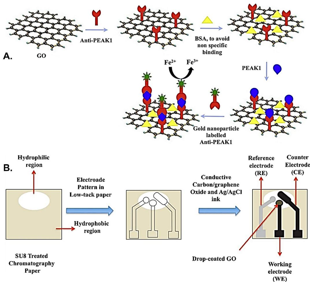
Fig. 8 A and B) Paper coated graphene oxide based immunosensor for pancreatic cancer biomarker (PEAK1 tyrosine kinase) detection. Figures A and B have been adapted from Prasad *et al.*, Sensors and Actuators B: Chemical, 2020.<sup>119</sup>
