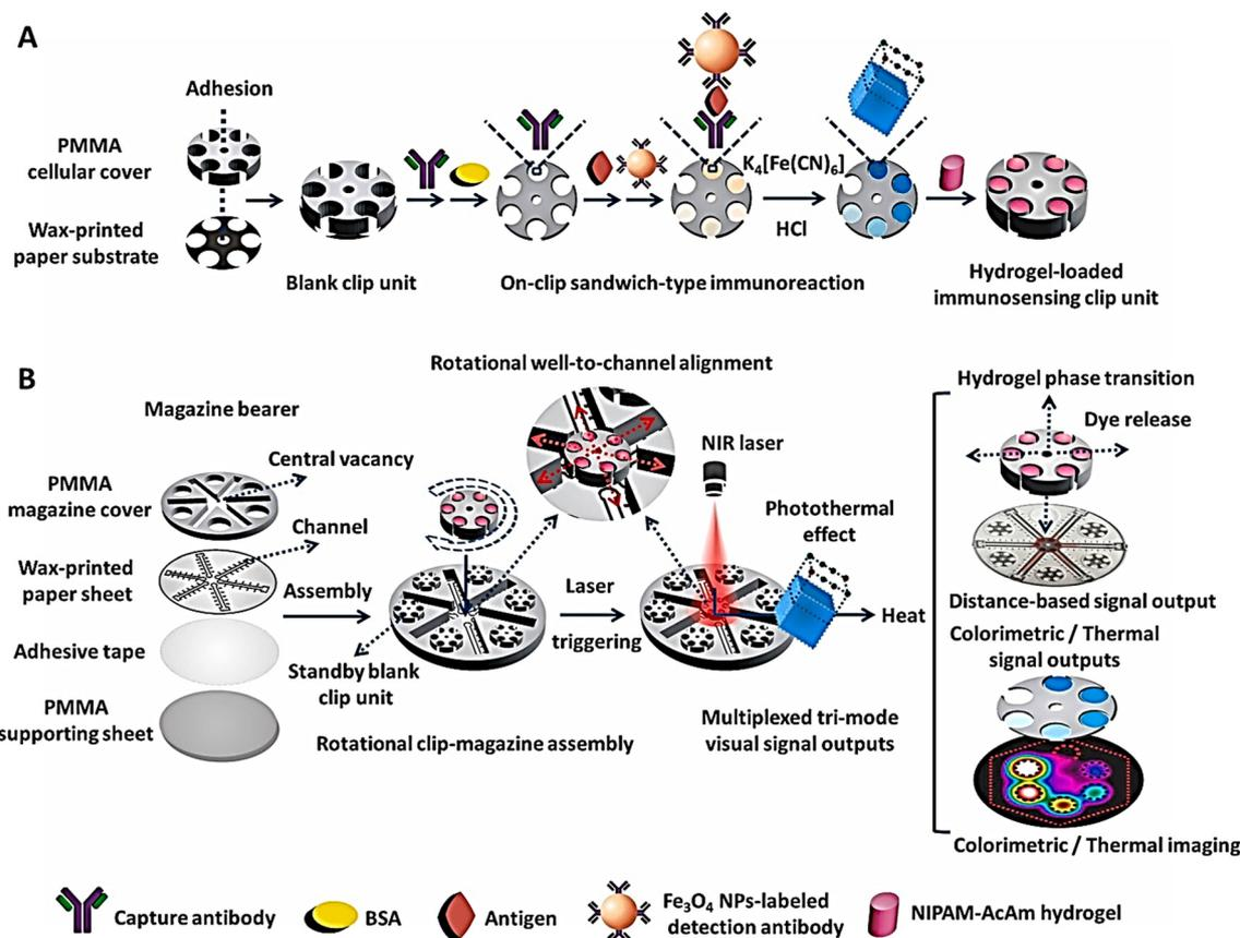
**Fig. 11** A) Development of photothermal responsive hydrogel loaded poly (methyl methacrylate)/paper hybrid disk (PT-disk) based sandwich immunosensor. B) Schematic representation of the clip and magnetic bearer assembly and tri-mode visual output of immunoassay signal from the PT-disk. Figures A and B have been adapted with permission from Fu *et al.*, *Biosensors and Bioelectronics*, 2020.<sup>174</sup>
