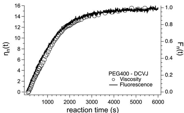
Fig. 17 Monitoring the synthesis of polyurethane (PU) in the presence of 9-(2,2-dicyanovinyl)julolidine (**DCVJ**). Relative viscosity variations ( $\eta_r(t)$ ) and relative fluorescence variations ( $F_r(t)$ ) are shown in open circles and a solid line, respectively.
