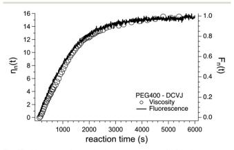
Fig. 17 Monitoring the synthesis of polyurethane (PU) in the presence of 9-(2,2-dicyanovinyl)julolidine (DCVJ). Relative viscosity variations  $(\eta_n(t))$  and relative fluorescence variations  $(F_n(t))$  are shown in open circles and a solid line, respectively.
