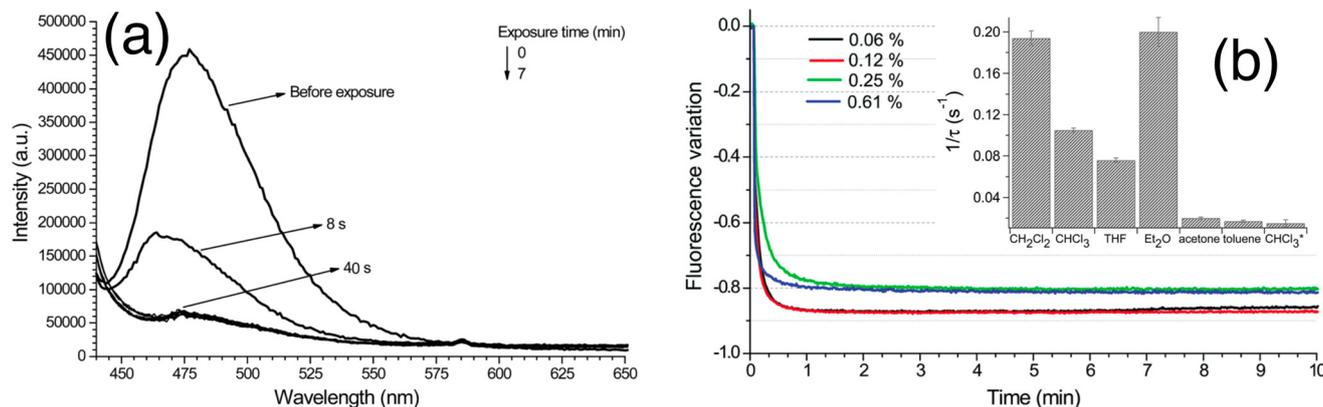
**Fig. 19** (a) Quenching of fluorescence emission of the P(STY-co-JCAEM) film (0.06 mol% JCAEM) as a function of exposure to chloroform vapors; (b) variation in the fluorescence maximum intensity with exposure time to chloroform vapors for all P(STY-co-JCAEM) (mol% of JCAEM) films; the inset shows the rate constant of the attenuation of emission intensity. Reprinted with permission from ref. 43. Copyright 2017. Royal Society of Chemistry.
