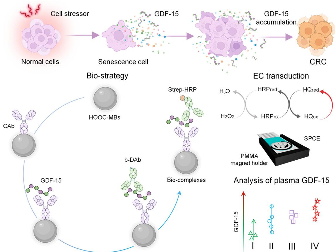
**Scheme 1** Schematic diagram showing the steps involved in the preparation of GDF-15 sandwich immunocomplexes on HOOC-MBs, the amperometric transduction of the resulting magnetic bioconjugates at a SPCE in the presence of H<sub>2</sub>O<sub>2</sub> and HQ, and the main application of the developed bioplatfrom. Created with Biorender.
