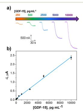
Fig. 2 Actual amperometric traces recorded at the indicated concentrations (a) and calibration graph (b) constructed for the determination of GDF-15 with the developed immunoplatform.
