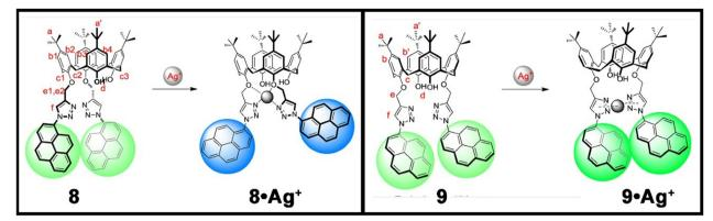
Fig. 6 The binding mechanism and 1:1 complex formation of probes 8 and 9 with Ag<sup>+</sup> ions (reprinted with permission from ref. 67. Copyright 2012. Elsevier).
