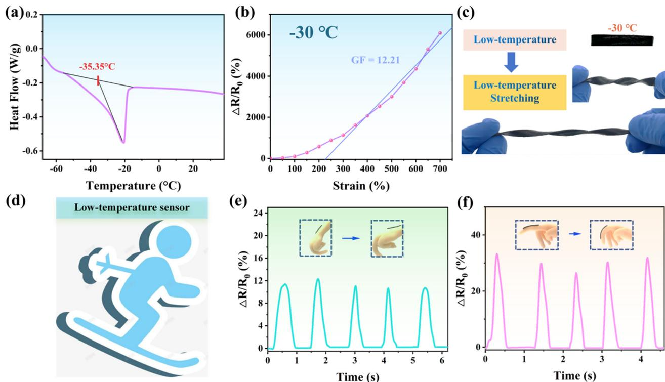
**Fig. 7** Anti-freezing property of the PAM organohydrogel-based strain sensor. (a) DSC curve in the temperature range of  $-70$ – $40$  °C; (b) resistance change-strain curve at  $-30$  °C; (c) photos of stretching sensor with and without EG at  $-30$  °C and  $20$  °C; (d) application scenario in low-temperature environment; response of the sensor attached to wrist (e) and finger (f) of a silicon at  $-30$  °C to the repeated bending.
