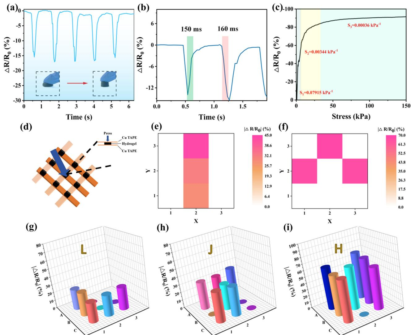
**Fig. 8** Demonstration of the PAA/starch/MXene organohydrogel-based pressure sensor. (a) Response to compressing and releasing; (b) response and recovery time; (c) relative resistance changes as a function of pressure; (d) sketch of  $3 \times 3$  array of pressure sensors; 2D pressure distributions of static loading (e and f); 3D pressure distributions of writing the letters 'L' (g), 'J' (h), and 'H' (i).
