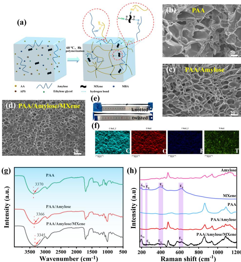
**Fig. 1** Fabrication and structural characterization of the organohydrogels. (a) Schematic of the synthesis process for PAA/starch/MXene organohydrogel; SEM images of (b) PAA, (c) PAA/starch, and (d) PAA/starch/MXene organohydrogels; (e) stretchability of the PAA/starch/MXene organohydrogel with knotted and twisted states; (f) elemental mapping images of C, O, F, and Ti elements in the PAA/starch/MXene organohydrogel; (g) FTIR spectra and (h) Raman spectra of the organohydrogels.
