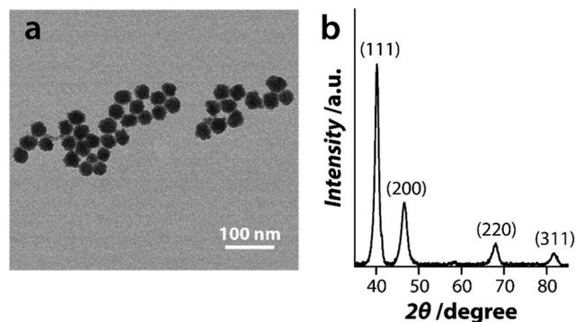
Fig. 1 Characterisation of PtNPs where (a) shows a representative TEM image of the nanoparticles and (b) shows their XRD pattern.
