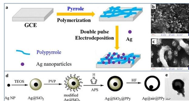
**Fig. 2** (a) Schematic diagram of the preparation of Ag/PPy/glassy carbon modified electrode; FESEM images of PPy (b) and Ag/PPy (c). Reproduced from ref. 63 with permission from Elsevier, copyright 2015. (d) Schematic diagram of the synthesis of the yolk-shell Ag@PPy nanoparticles. (e) TEM image of Ag@PPy yolk-shell nanoparticles. Reproduced from ref. 65 with permission from Elsevier, copyright 2010.
