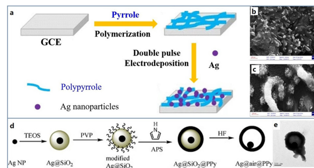
Fig. 2 (a) Schematic diagram of the preparation of Ag/PPy/glassy carbon modified electrode; FESEM images of PPy (b) and Ag/PPy (c). Reproduced from ref. 63 with permission from Elsevier, copyright 2015. (d) Schematic diagram of the synthesis of the yolk-shell Ag@PPy nanoparticles. (e) TEM image of Ag@PPy yolk-shell nanoparticles. Reproduced from ref. 65 with permission from Elsevier, copyright 2010.
