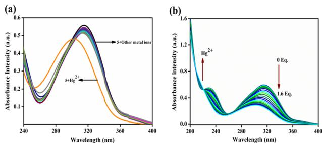
**Fig. 1** (a) The UV-visible absorption spectra of sensor 5 (2  $\mu\text{M}$ ) upon addition of different metal cations to  $\text{CH}_3\text{CN}/\text{H}_2\text{O}$  (8:2, v/v) solution. (b) Titration of sensor 5 (2  $\mu\text{M}$ ) with increasing concentration of  $\text{Hg}^{2+}$  ion (1 mM).
