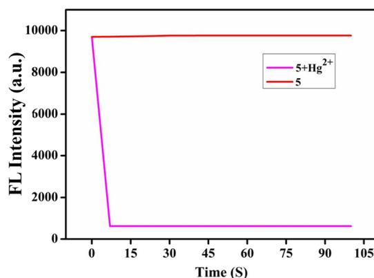
Fig. 5 Sensor 5 with  $\text{Hg}^{2+}$  ion response time.
