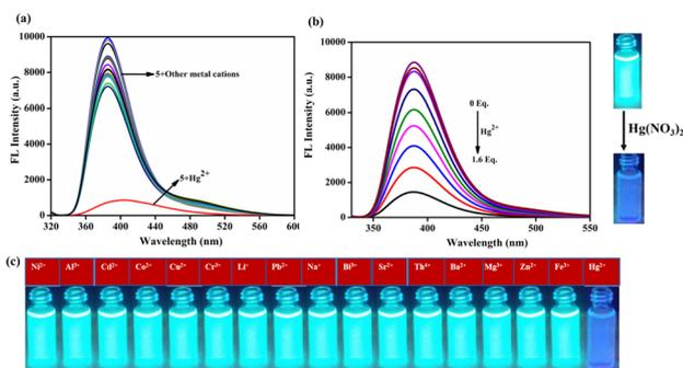
**Fig. 2** (a) Sensor 5 (2  $\mu\text{M}$ ) fluorescence spectra with different metal ions in  $\text{CH}_3\text{CN}/\text{H}_2\text{O}$  (8:2, v/v) solution. (b) Compound 5 (2  $\mu\text{M}$ ) was treated with different equivalents of  $\text{Hg}^{2+}$  ion (1 mM, 0 to 1.6 equivalents).
