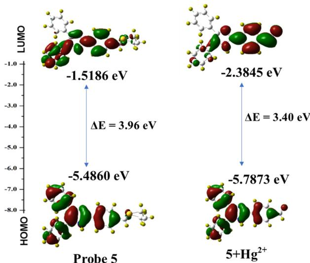
Fig. 7 HOMO and LUMO energy difference between 5 and 5 + Hg<sup>2+</sup>.
