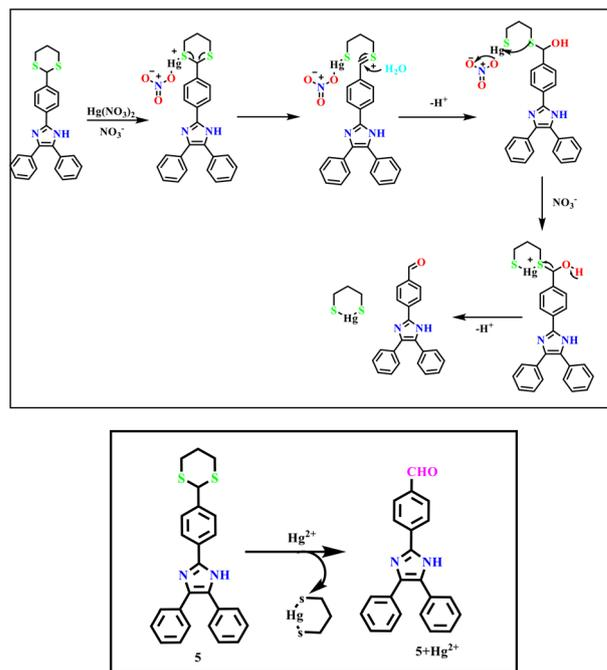
Scheme 2 Proposed mechanism for detecting  $\text{Hg}^{2+}$  by 5.
