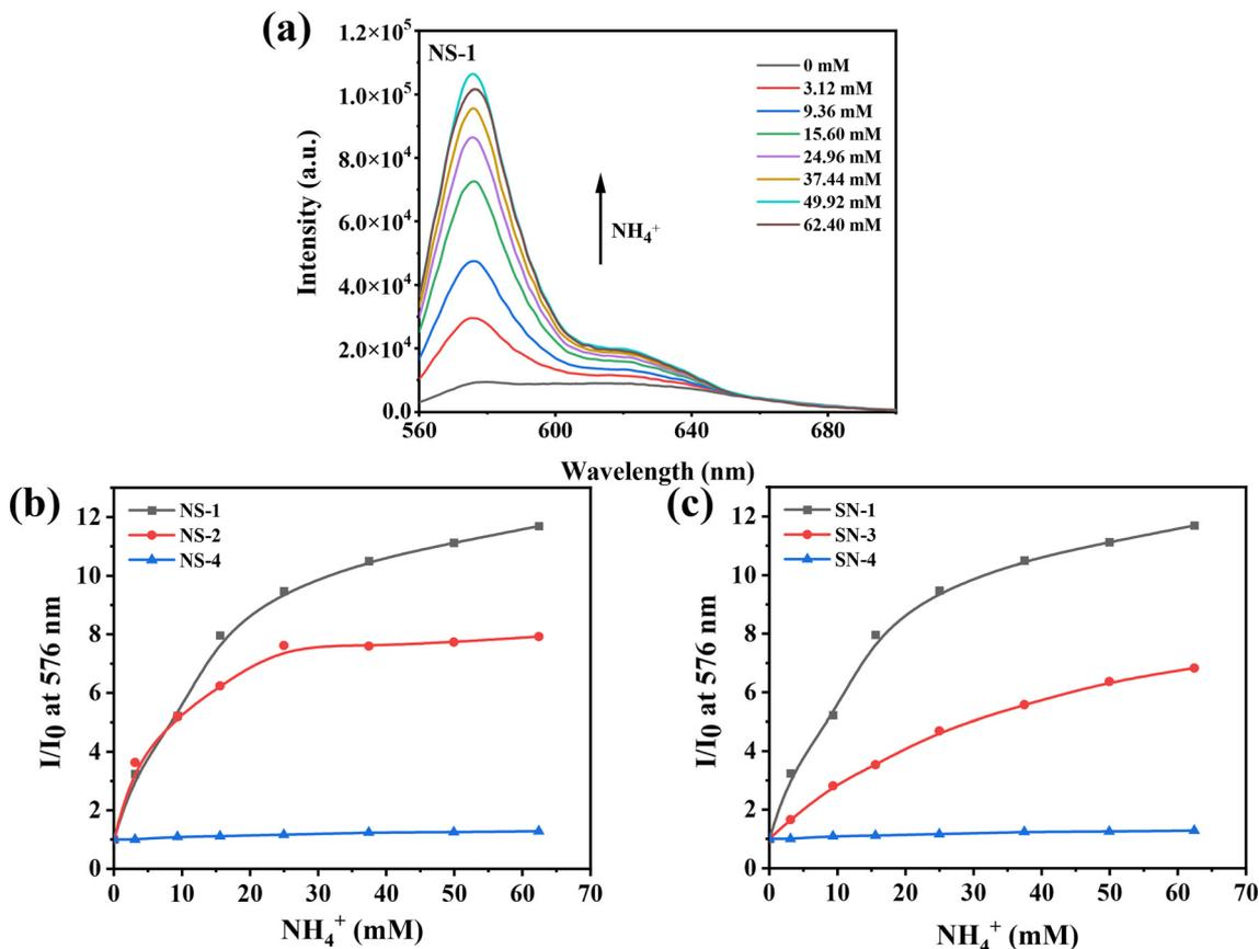
Fig. 2 Effects of buffer in the detection area on the sensor performance. (a) Emission spectra of the sensor NS-1 with buffer (1000 mM, pH = 6.5) at different  $\text{NH}_4^+$  concentrations. (b) Plots of the fluorescence intensity ratio ( $I/I_0$ ) at 576 nm against  $\text{NH}_4^+$  of sensors with different buffer capacities. (c) Plots of the fluorescence intensity ratio ( $I/I_0$ ) at 576 nm against  $\text{NH}_4^+$  of sensors containing buffers with different pH values.
