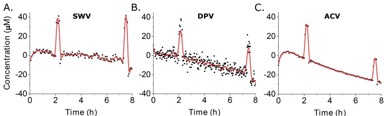
**Fig. 6** We calculated noise levels associated with each method (A: swv; B: DPV; C: ACV) as the root mean square deviation (RMSD) from the fitted data trends seen for our 37 °C whole blood studies (Fig. 5). The red curves represent the fitted estimate of the data, calculated from the average signals of four electrodes (black dots).
