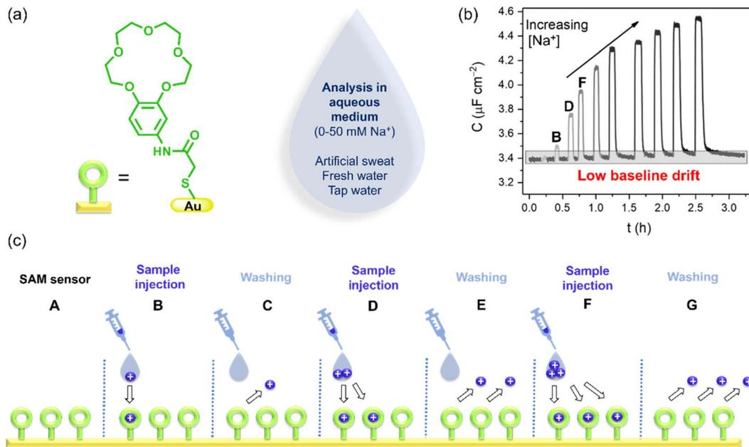
Fig. 1 (a) The receptor is a modified benzo-15-crown-5 that is immobilized on a gold electrode surface of a sensor for analysis of sodium ( $\text{Na}^+$ ) and other cations. (b) Non-faradaic capacitance response,  $C$ , of the surface-mounted receptor toward increasing  $\text{Na}^+$  concentrations. (c) Cartoon showing the ion binding and debinding process by the surface-immobilized receptor under continuous flow (reproduced from ref. 8 with permission from the Royal Society of Chemistry).
