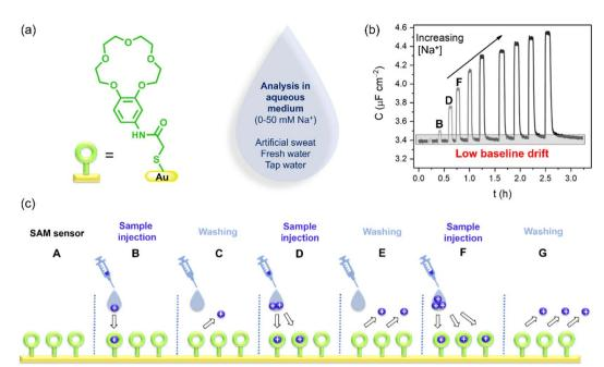
Fig. 1 (a) The receptor is a modified benzo-15-crown-5 that is immobilized on a gold electrode surface of a sensor for analysis of sodium (Na<sup>+</sup>) and other cations. (b) Non-faradaic capacitance response, *C*, of the surface-mounted receptor toward increasing Na<sup>+</sup> concentrations. (c) Cartoon showing the ion binding and debinding process by the surface-immobilized receptor under continuous flow (reproduced from ref. 8 with permission from the Royal Society of Chemistry).
