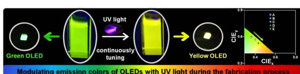
**The third strategy: modulating emission colors of organic light-emitting diodes with UV light during the device fabrication process**
