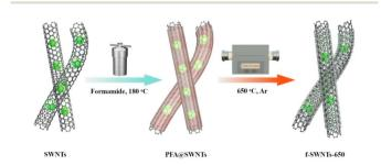
Scheme 1 Schematic illustration of the synthesis of the f-SWNTs-650 catalyst.
