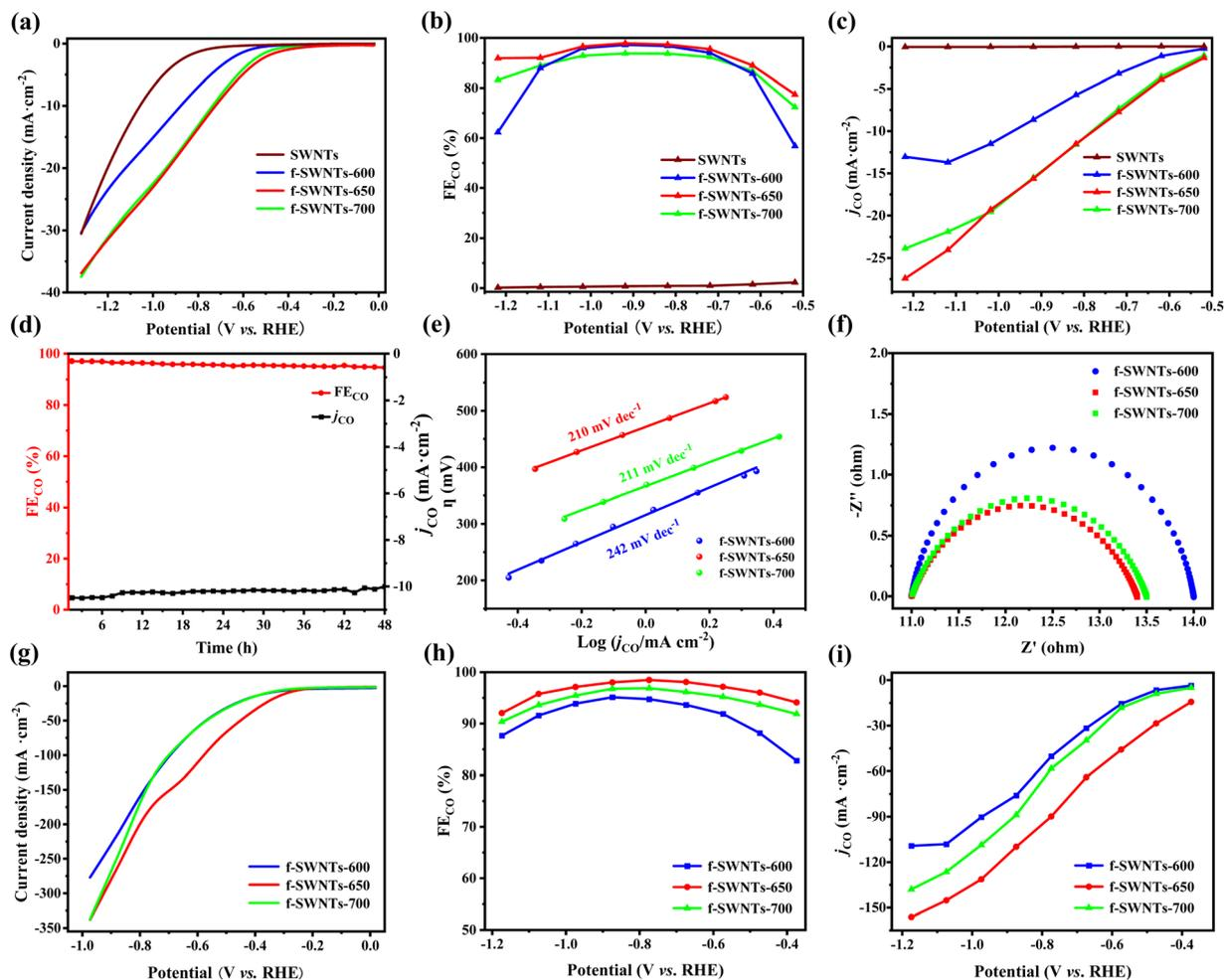
Fig. 3 In the H-type electrolytic cell: (a) linear sweep voltammetry curves, (b)  $FE_{CO}$  and (c) CO partial current density at different potentials, (d) long-term stability of the f-SWNTs-650 catalyst at  $-0.82$  V vs. RHE, (e) Tafel slope, and (f) Nyquist plots. In the flow cell: (g) linear sweep voltammetry curves, (h)  $FE_{CO}$  and (i) CO partial current density at different potentials.
