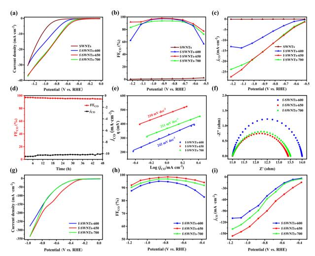
Fig. 3 In the H-type electrolytic cell: (a) linear sweep voltammetry curves, (b) FECO and (c) CO partial current density at different potentials, (d) long-term stability of the f-SWNTs-650 catalyst at -0.82 V vs. RHE, (e) Tafel slope, and (f) Nyquist plots. In the flow cell: (g) linear sweep voltammetry curves, (h) FE<sub>CO</sub> and (i) CO partial current density at different potentials.
