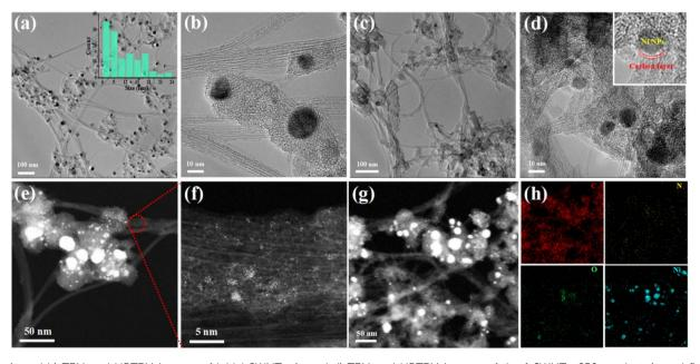
Fig. 1 (a and b) TEM and HRTEM images of initial SWNTs, (c and d) TEM and HRTEM images of the f-SWNTs-650 catalyst, (e and f) highresolution HAADF-STEM and (g and h) HAADF-STEM and the corresponding EDS images of the f-SWNTs-650 catalyst.
