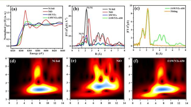
Fig. 2 (a) XANES spectra at the Ni K-edge, (b) Fourier transformed (FT)  $k^3$ -weighted  $\chi(k)$ -function of the EXAFS spectra for Ni foil, NiO, SWNTs and f-SWNTs-650, (c) EXAFS fitting curves of the f-SWNTs-650 catalyst at R space (inset showing the schematic model) and (d-f) WT for the  $k^3$ -weighted EXAFS signals of Ni foil, NiO and the f-SWNTs-650 catalyst.
