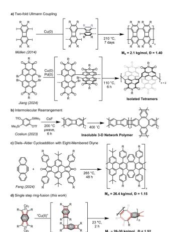
Fig. 1 (a) Ullmann coupling of aryl halides to yield planar eightmembered rings and tub-shaped COT-containing tetramers; (b) benzyne dimerization to yield COT-containing network polymers; (c) Diels–Alder cycloaddition of diyne and bis-cyclopentadienone,  $M_{\rm n}$  and D were determined after purification by recycling SEC; (d) dimerization of bis-zirconacycles.
