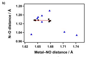
Fig. 6 (a) Plot of the N–O bond distance (Å) against the N–O bond stretching frequency (cm $^{-1}$ ) for {MnNO} $^6$  and {FeNO} $^6$  complexes. (b) Plot of the N–O bond distance (Å) against the M–NO bond length (Å). Triangle (blue) and rectangle (black) represent {MnNO} $^6$  and {FeNO} $^6$  complexes, respectively. The solid red line shows a least-squares linear fit of the data.
