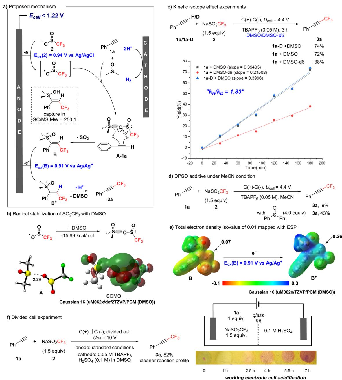
Scheme 3 Proposed mechanism with supporting experimental evidence.
