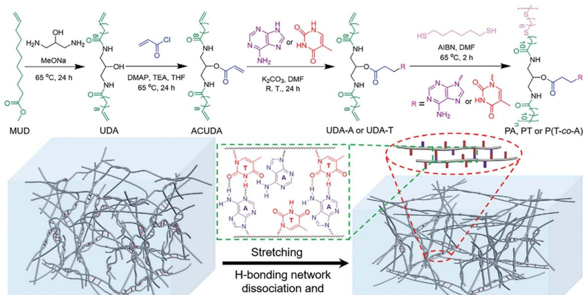
Fig. 9 Synthesis of nucleobase-containing polymers and the dissociation and reorganization of hydrogen-bonding networks of nucleobase-containing flexible long-chain copolymers under elongation.<sup>100</sup> Adapted from ref. 100 with permission from Wiley-VCH, copyright 2022.
