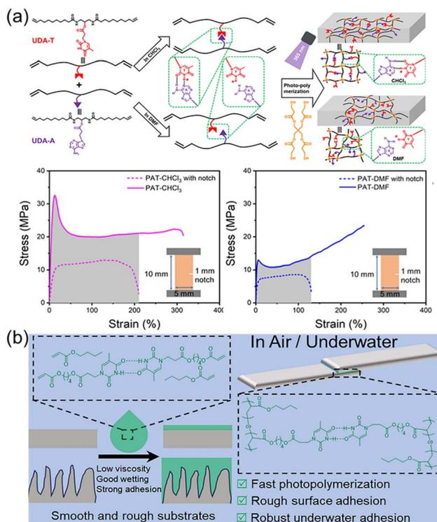
Fig. 7 (a) Schematic representation of the nucleobase-containing networks made in the presence or absence of selective hydrogen bonds.<sup>101</sup> Adapted from ref. 101 with permission from American Chemical Society, copyright 2024. (b) Schematic illustration showing efficient adhesion on smooth and rough surfaces through utilizing the hydrogen bonds of nucleobases.<sup>107</sup> Adapted from ref. 107 with permission from Royal Society of Chemistry, copyright 2024.
