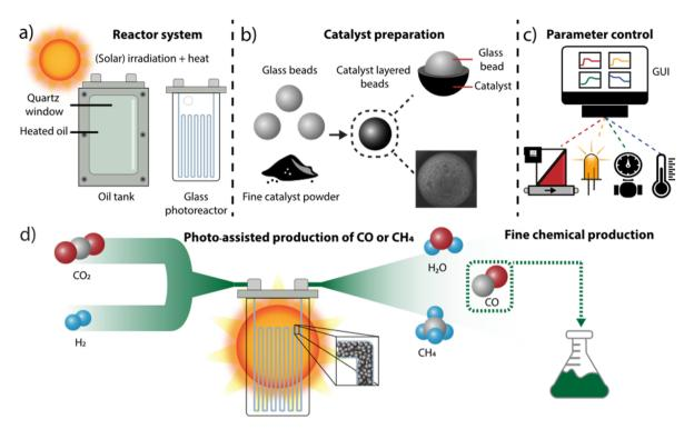
Fig. 1 (a) Principles of the modular system, including the heating and the photoreactor. (b) Schematic representation of the catalyst loading on glass beads, with a cross section and SEM image. (c) Overview of the automated control system for the individual flow rate, light intensity, pressure and temperature. (d) Scheme for the production of fine chemicals from carbon dioxide and hydrogen.
