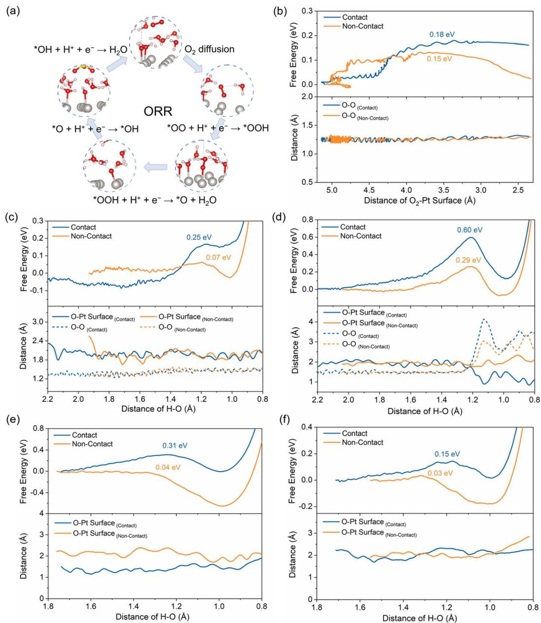
Fig. 3 In the contact and non-contact structures, the diagram of the ORR elementary step pathway (a) and the evolution of free energy and bond lengths for each elementary step: (b)  $O_2$  diffusion; (c)  $*OO + H^+ + e^- \rightarrow *OOH$ ; (d)  $*OOH + H^+ + e^- \rightarrow *O + H_2O$ ; (e)  $*O + H^+ + e^- \rightarrow *OH$ ; (f)  $*OH + H^+ + e^- \rightarrow H_2O$ .
