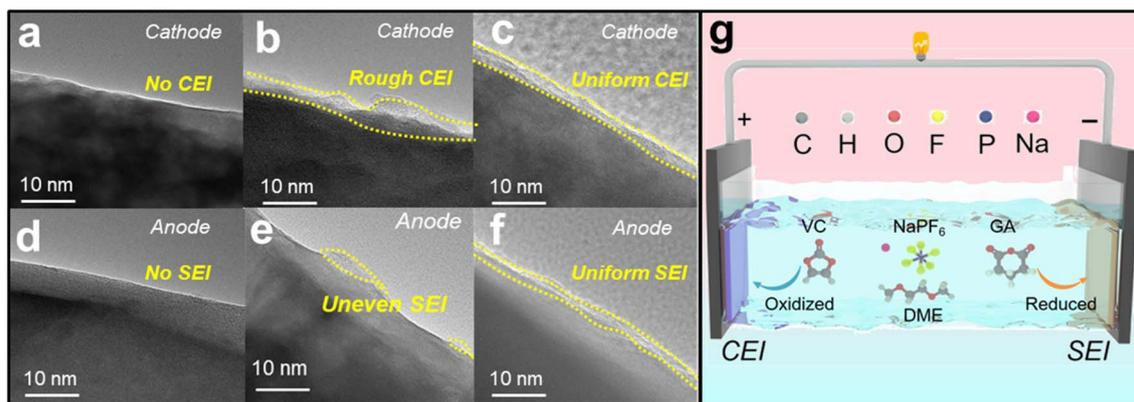
Fig. 6 The mechanism analysis of electrolytes. HRTEM images of NVP in (a) 1 M NaPF<sub>6</sub> + DME, (b) 1 M NaPF<sub>6</sub> + DME/VC and (c) 1 M NaPF<sub>6</sub> + DME/VC + 2 wt% GA electrolytes. HRTEM images of HC in (d) 1 M NaPF<sub>6</sub> + DME, (e) 1 M NaPF<sub>6</sub> + DME/VC and (f) 1 M NaPF<sub>6</sub> + DME/VC + 2 wt% GA electrolytes. (g) The illustration of film formation on the cathode and anode in 1 M NaPF<sub>6</sub> + DME/VC + 2 wt% GA electrolyte.
