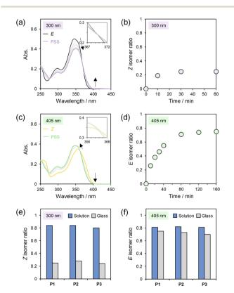
Fig. 6 UV/vis absorption spectra of (a) E-P1 thin film upon 300 nm irradiation and (c) Z-P1 thin film upon 405 nm irradiation. Z and E isomer ratios determined from  $^1H$  NMR spectra in the photo-isomerization of (b) E-P1 and (d) Z-P1 thin films. Summary of Z and E isomer ratios determined from  $^1H$  NMR spectra at (e) 300 nm and (f) 405 nm PSSs in THF solution and in the glassy state of P1, P2, and P3.
