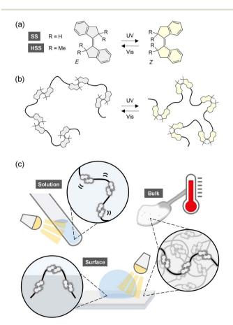
Fig. 1 (a) Photoisomerization of SS and HSS. (b) Conformational changes of a single polymer chain by photoisomerization of the mainchain HSS. (c) Overview of this study.
