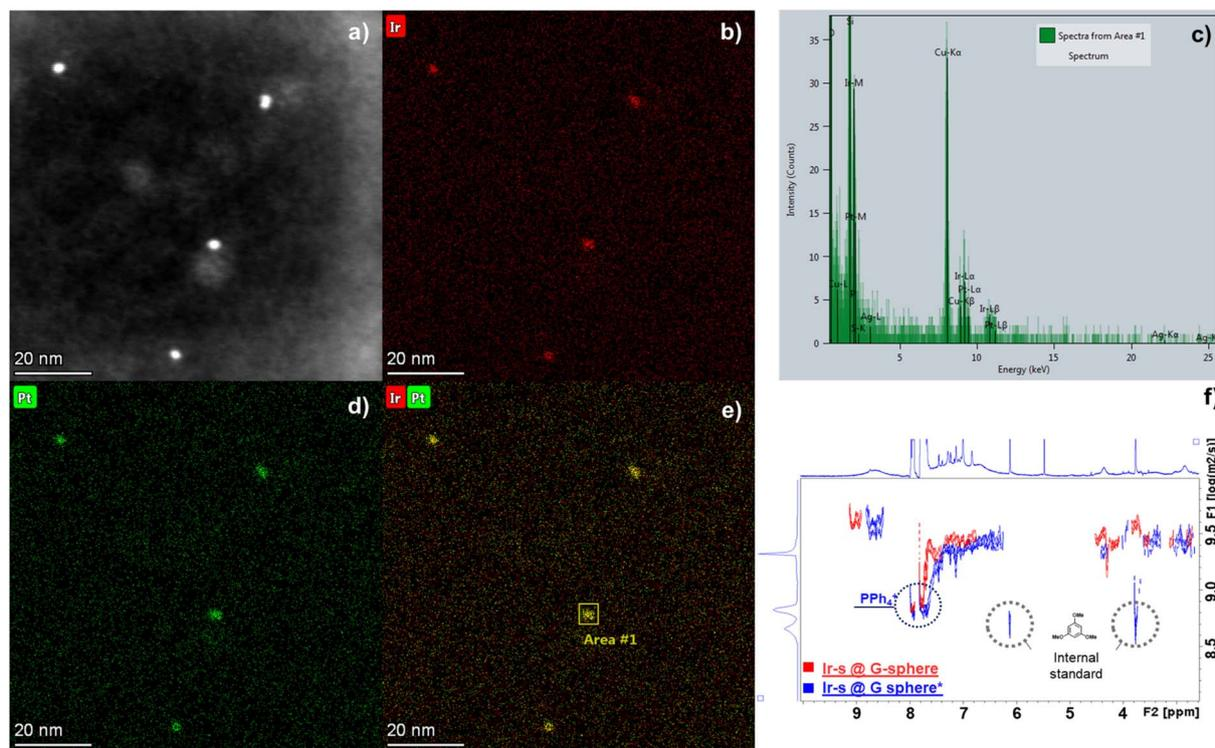
Fig. 4 (a) HAADF-STEM image of Ir-s@G-sphere\* and corresponding EDX maps of (b) Ir, (d) Pt and (e) an overlay of Ir and Pt, (c) EDX pattern of the selected area in (e), (f)  $^1\text{H}$ -DOSY-NMR overlay of Ir-s@G-sphere\*/before (red) and Ir-s@G-sphere\*/after hydrogenation.
