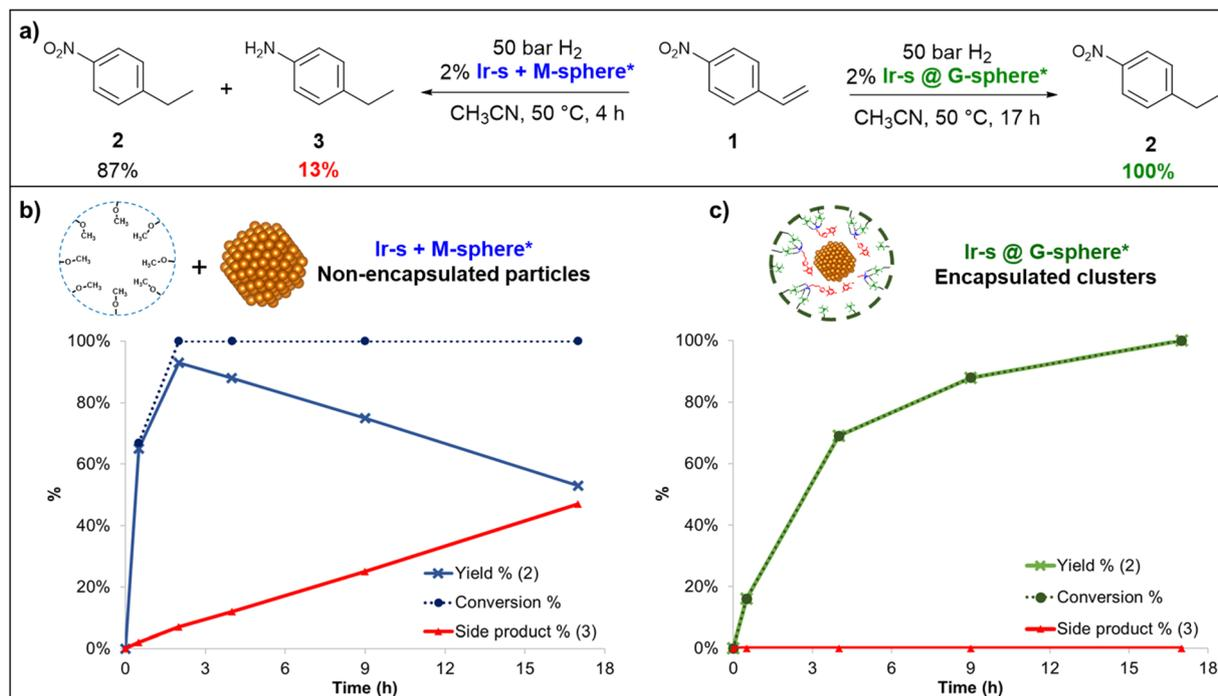
Fig. 5 (a) Hydrogenation of 4-nitrostyrene (1): product composition at full conversion in the presence of Ir-s + M-sphere\* (left) and Ir-s@G-sphere\* (right), (b) hydrogenation of 1 over time in the presence of Ir-s + M-sphere\* and (c) in the presence of Ir-s@G-sphere\*. ([1] = 60 mM in CH<sub>3</sub>CN, 2% Ir vs. 1).
