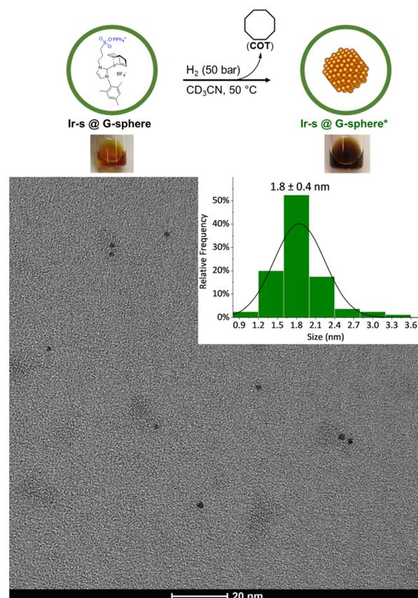
Fig. 2 Top: nanocluster synthesis conditions and representative images of the solutions of **Ir-s@G-sphere** before and after hydrogenation (**Ir-s@G-sphere\***) respectively. Bottom: representative TEM image of **Ir-s@G-sphere\*** and corresponding size distribution (in diameter).
