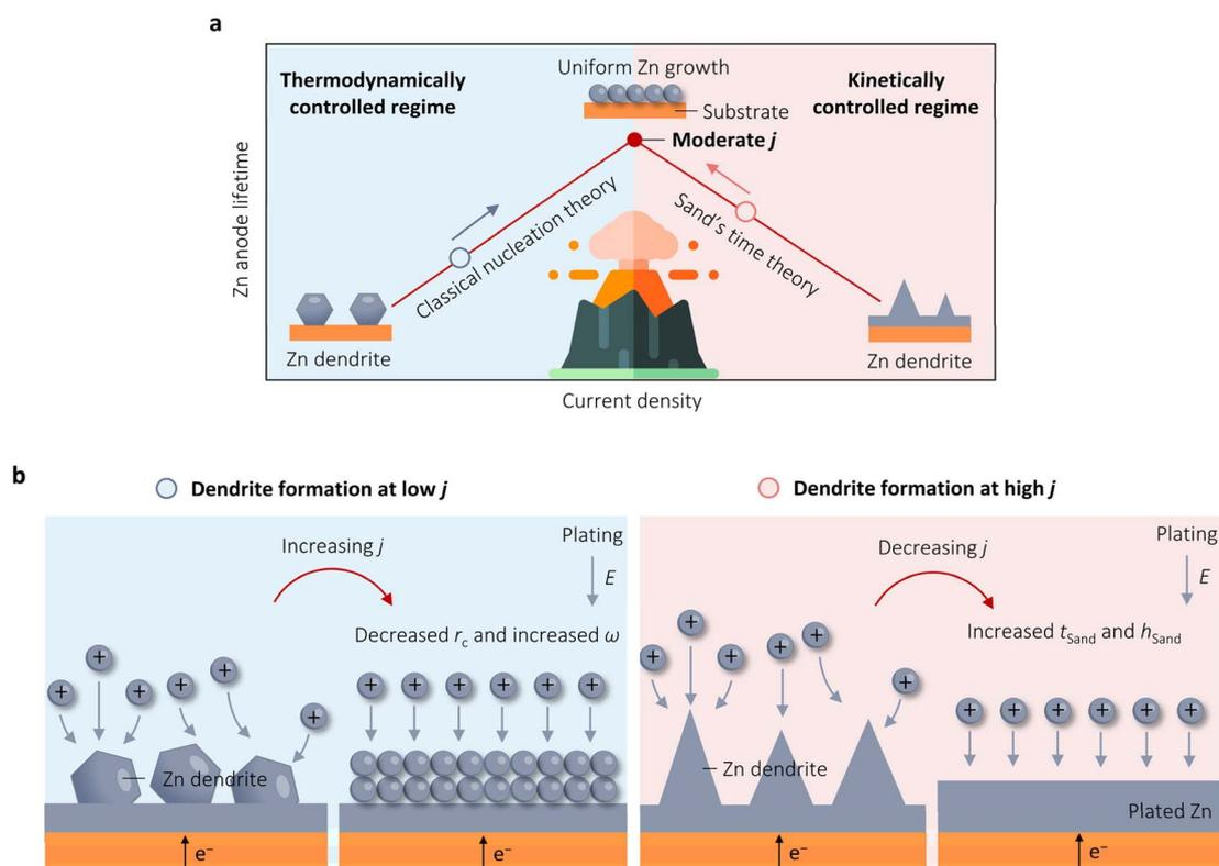
Fig. 4 Beneficial thermodynamic and adverse kinetic characteristics of  $j$  on Zn stability. (a) Illustration of the variation in the cycling lifetime of Zn anodes as  $j$  increases, which is governed by different mechanisms. (b) Schematic illustration of the protocol to improve the lifespan of Zn anodes through regulating  $j$ .
