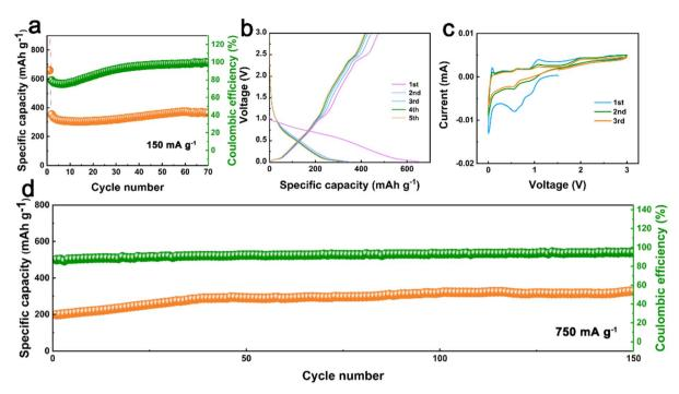
Fig. 4 (a) The cyclic performance of CityU-26 at 150 mA  $g^{-1}$ , (b) charge–discharge voltage profiles of the first 5 cycles under 150 mA  $g^{-1}$ , (c) CV curves at 0.1 mV  $s^{-1}$ , (d) cyclic performance at 750 mA  $g^{-1}$  of CityU-26 as a SIB anode.
