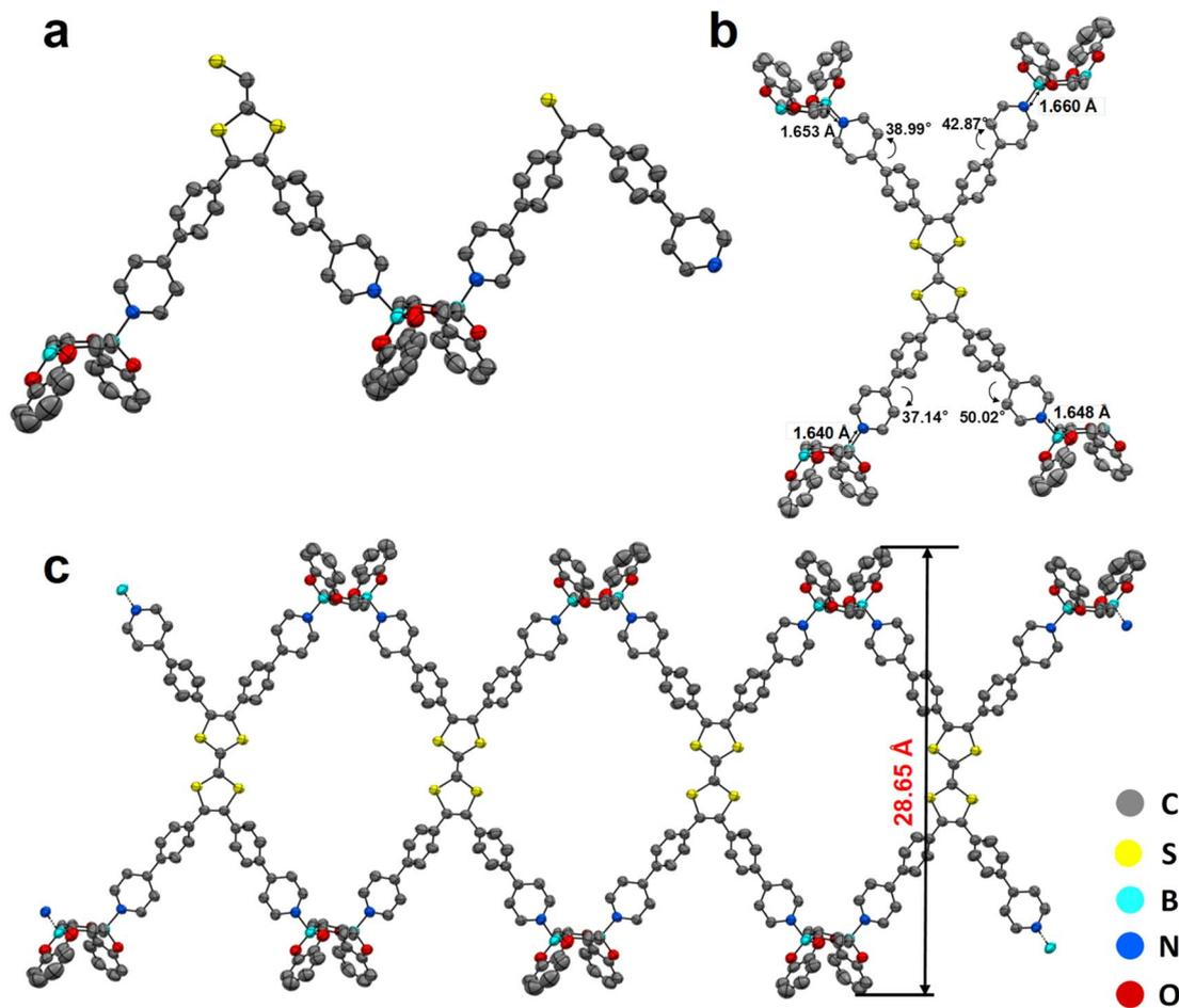
Fig. 2 (a) The asymmetric unit of **CityU-26**. Thermal ellipsoids are drawn at the 50% probability level. Hydrogen atoms and toluene molecules are omitted for clarity. The yellow, red, blue, and cyan balls represent sulfur atoms, oxygen atoms, nitrogen atoms, and boron atoms, respectively. (b) TTF-py monomer and the four BACT units to which it is connected in **CityU-26**. (c) A single nanobelt with a thickness of 28.65 Å in **CityU-26**.
