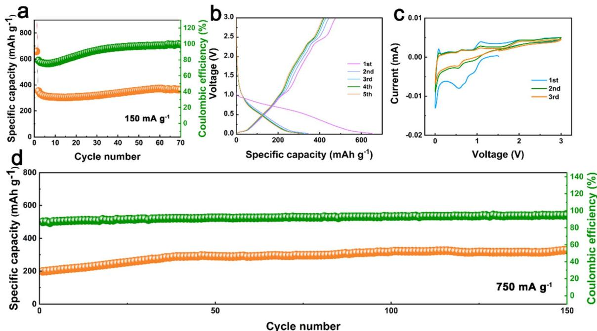
Fig. 4 (a) The cyclic performance of CityU-26 at  $150 \text{ mA g}^{-1}$ , (b) charge–discharge voltage profiles of the first 5 cycles under  $150 \text{ mA g}^{-1}$ , (c) CV curves at  $0.1 \text{ mV s}^{-1}$ , (d) cyclic performance at  $750 \text{ mA g}^{-1}$  of CityU-26 as a SIB anode.
