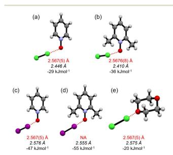
Fig. 5 The DFT structures of (a)  $\rm Cl_2$ -PyNO (b)  $\rm Cl_2$ -26DiMePyNO, (c)  $\rm I_2$ -PyNO (d)  $\rm I_2$ -26DiMePyNO and (e)  $\rm Cl_2$ -dioxane optimized at the PBE0-D3/def2-TZVP level of theory. Red broken lines represent XBs. The red font represents XB distances of the crystal structure and the italicized black font represents XB distances of DFT optimized structures. NA: crystal structure is not available.
