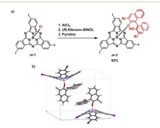
Fig. 2 (a) Synthetic scheme for the preparation of m-3 as a mixture of diastereomers from racemic m-1 via activation of the axial position with AlCl<sub>3</sub>. (b) Asymmetric unit of the crystal structure of m-3 showing the presence of two diastereomeric species. Toluene molecule of crystallization has been omitted for clarity.
