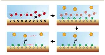
4 Proposed mechanism for simultaneous generation of hydrogen and hydroxyl radicals caused by water-solid contact electrification.
