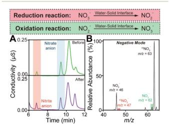
Fig. 2 (A) Ion chromatography showing the transformation of  $NO_2^-$  and  $NO_3^-$  before and after the water–solid contact. (B) Mass spectrum in negative mode showing the oxidation of  $NO_2^-$  and the reduction of  $^{15}NO_3^-$ .
