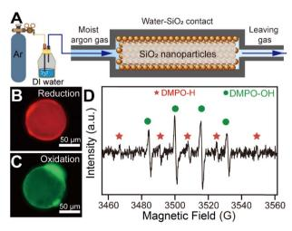
Fig. 1 (A) Schematic representation of the experimental setup. (B) A typical fluorescence microscopy image of reductive species generated on the surface of a  $SiO_2$  microsphere. (C) A typical fluorescence microscopy image of ROS generated on the surface of a  $SiO_2$  microsphere. (D) Corresponding ESR result for  $SiO_2$  micro-spheres after contacting with water-carrying argon gas.
